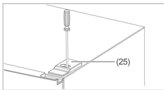
7. Screw the cover (25) onto the opposite side tightly.
