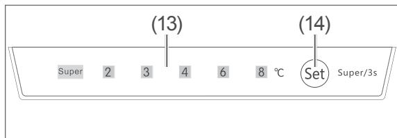
Use the temperature controller (13) to set the temperature in the fridge.
