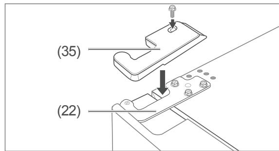
6. Screw down the protective cover (35) tightly.
