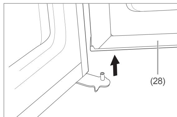
8. Open the freezer door (28), remove it and place it to one side.
