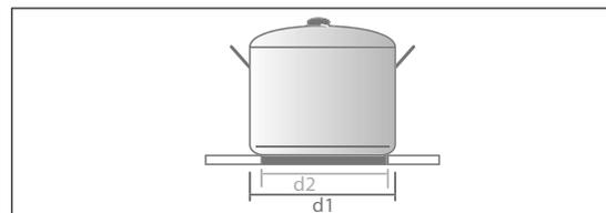
The diameter **d1** is always given for saucepan and pan size. **d2** base diameter is always around 2 cm smaller. Pots that are too big can cause paintwork damage.
