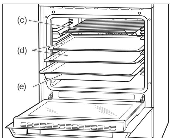
The supplied baking trays (d) and the dripping pan (e) have an angled edge. Please ensure that this edge is facing forward on being placed in the oven. The grilling rack (c) must be inserted as shown.
