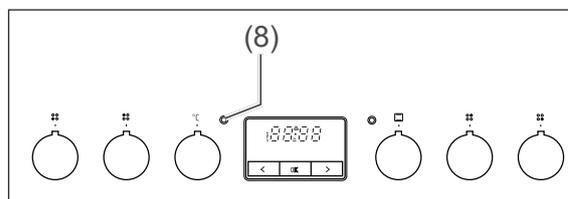
The red oven light (8) will illuminate as soon as you have selected a heating method and set the temperature. It will light up while the oven is heating up and/or re-heating. Once it goes out, the set oven temperature has been reached.
