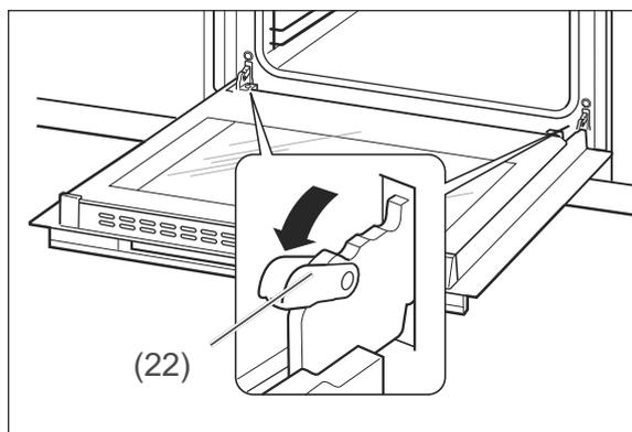
2. Fold the clips (22) on both sides all the way forward. Use a screwdriver if necessary.
