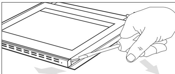
2. Remove both screws that secure the top metal grid.
