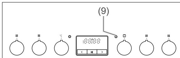
The yellow power indicator light (9) is illuminated as soon as one cooking zone or the oven is switched on. It will switch off again when **all** of the cooking zones **and** the oven are switched off.
