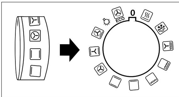
Use the function switch (12) to switch on the oven and select the heating method. The oven light will turn on.
