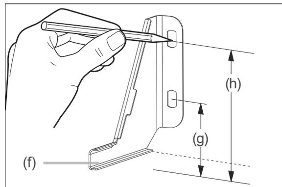
4. Position the tilt protection (f) on the line on the wall such that the side with the holes lies flat against the wall and the protruding limb fits into the slot on the cooker.
