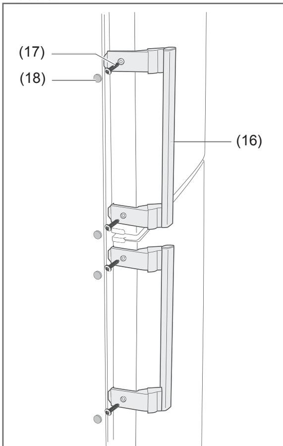
2. Attach the door handles (16) to both doors using the enclosed screws (17).
