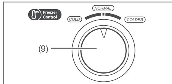
You can use the temperature controller (9) to set the temperature in the freezer, depending on the ambient temperature (e.g. higher in summer and lower in winter).
