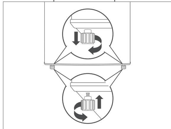
3. Level out any unevenness on the ground using both of the front screw feet.
