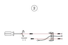
Drill holes & apply plastic anchors With screws
