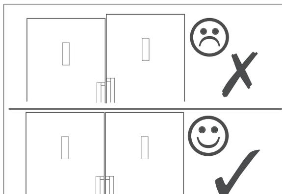
1. Place the two appliances next to each other and use the screw feet on each appliance to ensure that they are both positioned at the same height.
