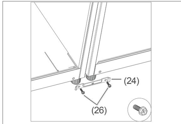
6. Then connect the appliances at the front using the connecting piece for the front of the appliance (24) and two of the screws (26).
