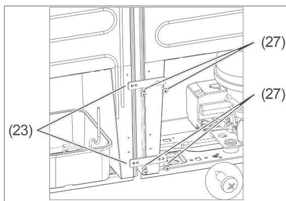
2. First, connect the appliances using two of the connecting pieces (23) and four of the screws (27).
