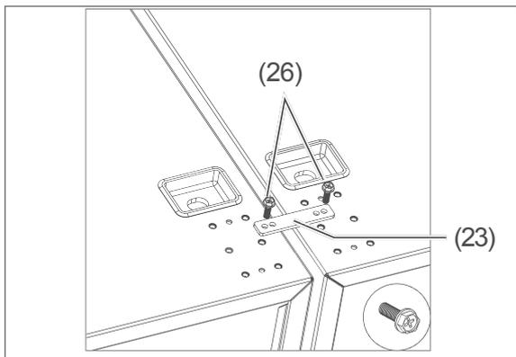
4. Use the third connecting piece (23) and two of the screws (26) to connect both appliances.
