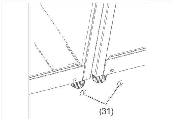
5. Use a string or a small screwdriver to remove the blind plugs (31) on the front of the appliances.
