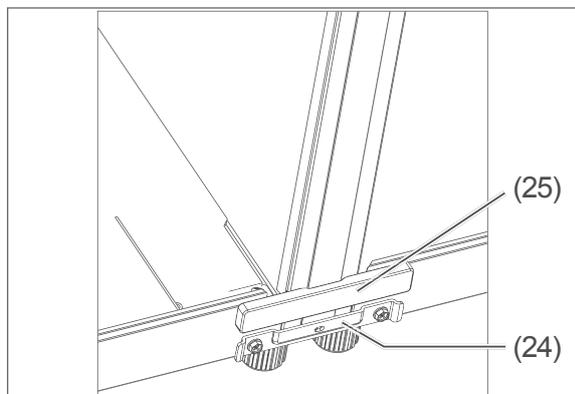
9. Attach the cover panel (25) for the connecting piece for the front of the appliance (24).
