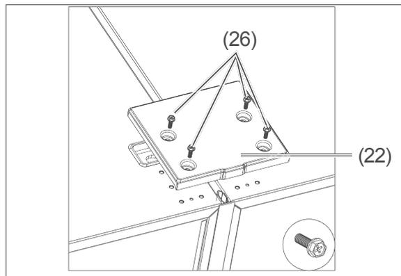
8. Screw down the upper cover (22) with the four remaining screws (26).
