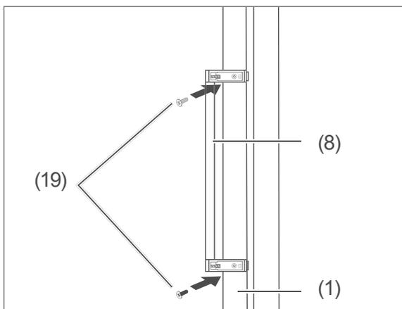
2. Screw the door handle (8) to the appliance door (1) using the screws provided (19).
