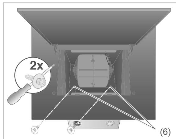
6. Screw two fixing screws to secure the Exhaust hood through the securing opening (6) into the prepared dowels and screw the Exhaust hood to the wall.
