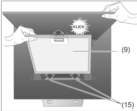
5. Once the grease filter is fully dry, insert it with the pins into the openings (15).
