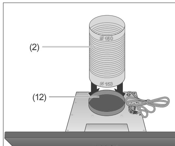
3. Place the exhaust air hose (2) with the 153 mm diameter opening onto the exhaust air opening (12).
