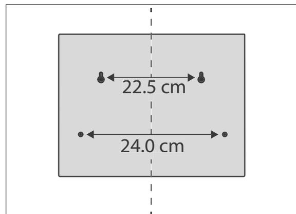
3. To maintain the lateral distances, mark the four drill holes on the wall according to the diagrams above.
