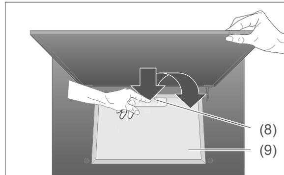
5. Slide the lock (8) of the grease filter (9) to the side and carefully remove the grease filter.
