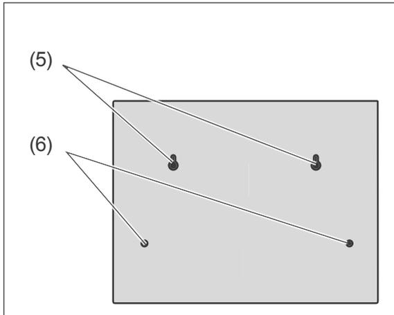
1. Screw 2 fixing screws into the upper screw plugs so that both screws are protruding about 1 cm.
