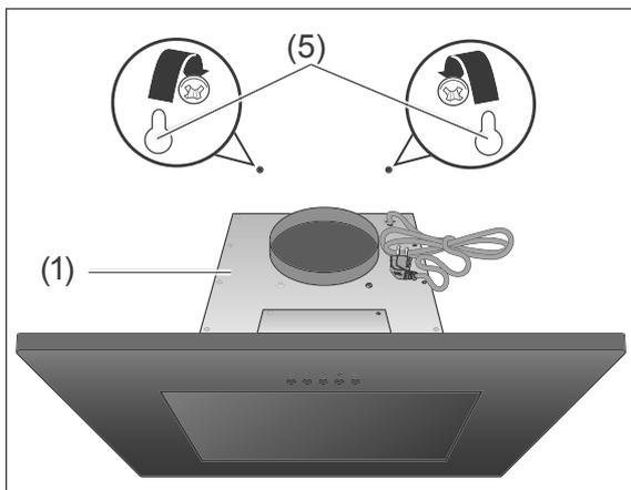
3. If necessary, remove the Exhaust hood again and loosen or tighten the screws in order to ensure that it is flush with the wall.
