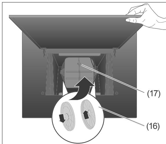
5. Place the new charcoal filters to the right and left of the motor and tighten them in an anti-clockwise direction. Allow the lock to click into place.
