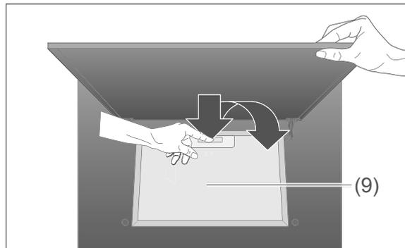
3. Slide the lock of the grease filter (9) side-ways and carefully remove the grease filter.
