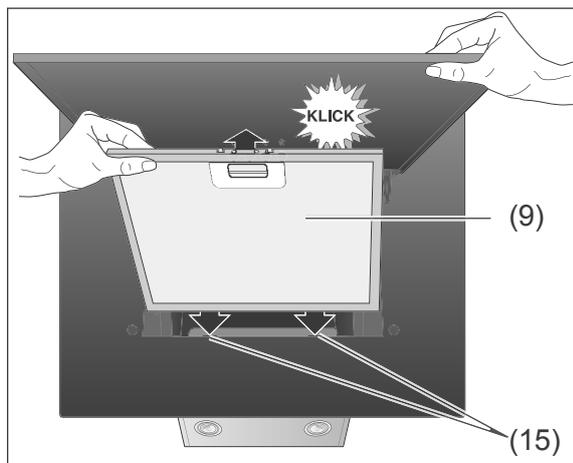
6. Place the grease filters (9) with the pins into the openings (15).
