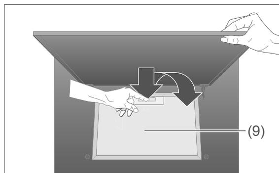
3. Slide the lock of the grease filter (9) sideways and carefully remove the grease filter.
