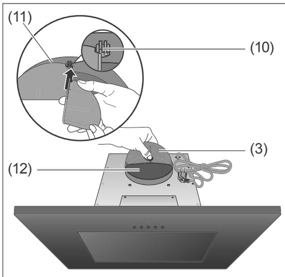
1. Insert the two wings of the check valve (3) using the pins (10) into the mounting holes (11) of the exhaust port (12). Gently bend the wings a little so as not to break off the sensitive plastic noses.
