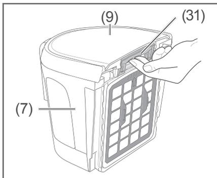
4. Release the locking mechanism (31) under the dust bin lid (9) and remove the dust bin (7).
