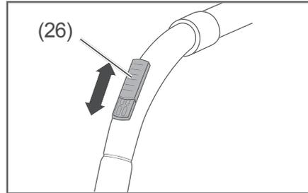
You can adjust the suction force as needed by using the air by-pass vent (26). The covering of the air by-pass vent (26) can be adjusted as desired.
