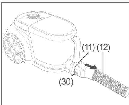
2. Pull the suction hose (12) out of the opening (11) of the suction hose connection. First press the locking mechanism (30) and then remove the suction hose (12).
