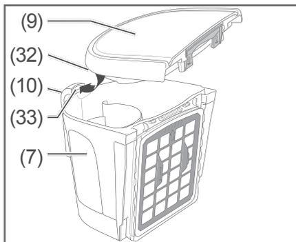
6. Place the dust bin lid (9) back onto the dust bin. Make sure that the mounting bracket (32) on the dust bin lid (9) clicks into the opening (33) on the dust bin (10) handle (7).
