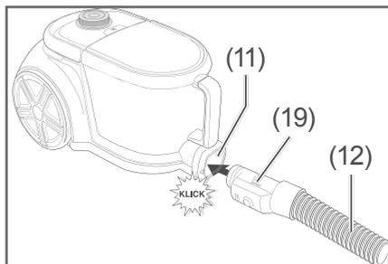
2. Put the suction hose (12) with the connector (19) in the opening (11) for the suction hose connection.
