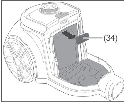
3. Remove the coarse dust filter (34) as illustrated.
