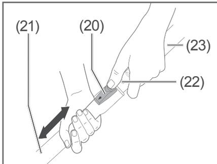
4. The length of the telescopic tube (13) can be adjusted to suit the height of its user. To do this, hold the upper part (23) of the telescopic tube (13) with one hand and press the locking mechanism (20) downwards. At the same time, use your other hand to push the lower part (21) of the telescopic tube (13) away from or towards you. Make sure that the lower part (21) of the telescopic tube (13) audibly clicks into one of the notches (22) in the upper part (23) of the telescopic tube (13).
