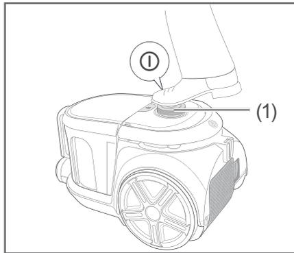
3. Use your foot to operate the on/off foot switch (1), to switch the appliance on.
