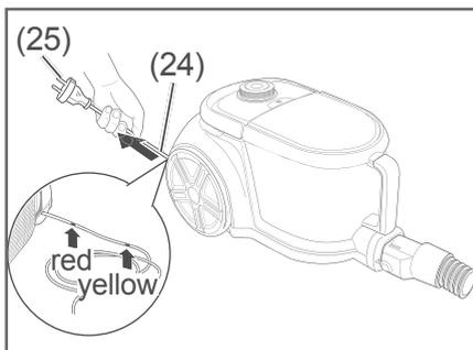
1. Pull the mains cord (24) out by the mains plug (25) until the yellow marking is visible on the mains cord (24).
