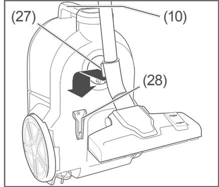
1. Use the handle (10) for the dust bin to lift the appliance and position it upright.
