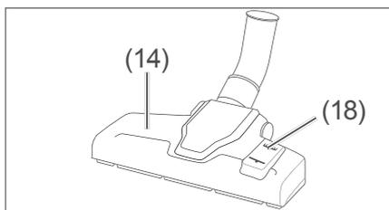
You will work with the floor nozzle (14) most of the time as it is designed for large, flat surfaces.
