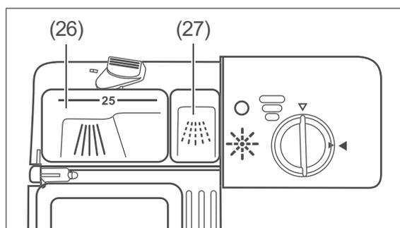
2. The large compartment (26) is the main wash compartment; the small one (27) is the pre-wash compartment.
