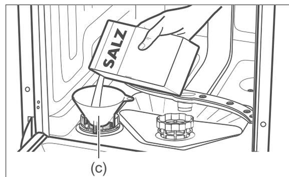
4. Place the supplied filling funnel (c) on the compartment opening.
