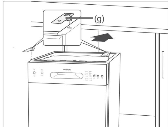
2. Insert the two mounting brackets (g) into the front slots on the top of the dishwasher so that you can screw the dishwasher to the worktop subsequently.
