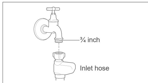
For water supply, you need a water tap with a 3/4 inch screw connector.
