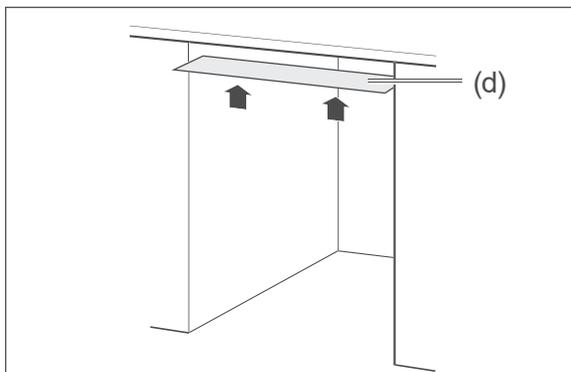
1. To protect the worktop against condensation, affix the enclosed protective film (e) to the underside of the worktop. This will help you minimise damage to the worktop from the outflow of hot steam.
