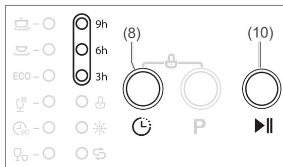
1. Press the “Delayed start” button (8) repeatedly until the LED to the left of the desired delay lights up.
