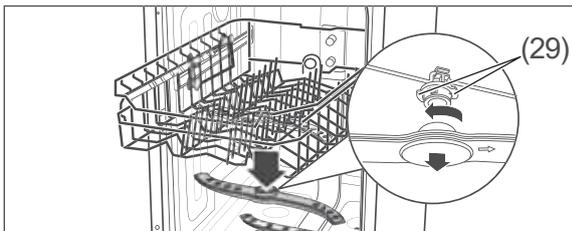
3. The upper spraying arm is affixed using a bayonet closure. To remove the spraying arm, hold the two serrated bayonet grips (29) still and turn the spraying arm clockwise.
