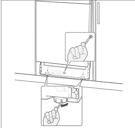
6. The height of both front feet and the back foot of the appliance can be adjusted to align the dishwasher horizontally. The front feet are equipped with slots. Insert a screwdriver into one of the slots and use it to turn the appliance feet to the desired height.
