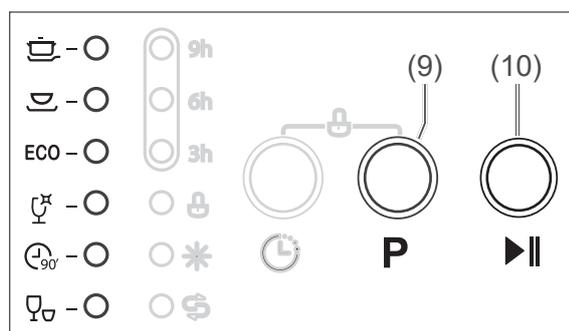
2. Press the **P** button (9) repeatedly until the LED to the right of the desired programme symbol lights up.
