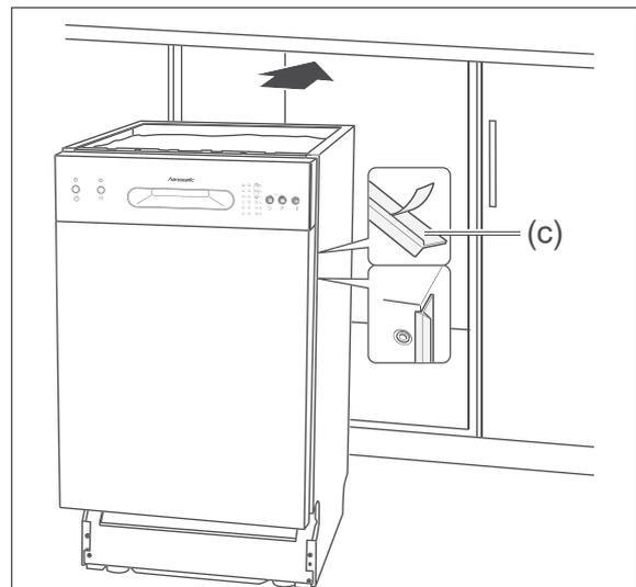
3. Remove the protective films from the side end profiles (c).
