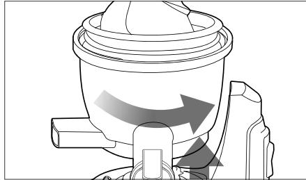
4. Remove the juicing screw, strainer and rotation wiper unit from the juicing bowl. Clean with provided brush.
