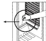
Make sure that the drain gully and the drain opening are not blocked so that the water produced in the refrigerator can always flow off unobstructed.
