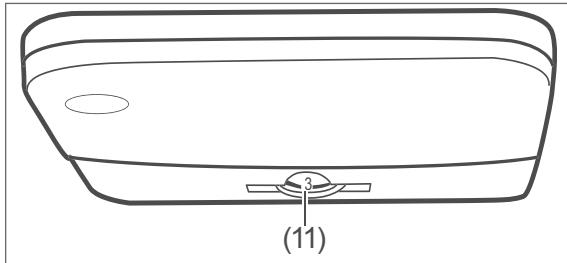
The temperature controller (11) is also used to switch the appliance on and off. It is at the top in the fridge.
