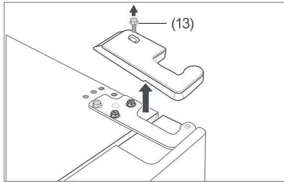
2. Unscrew the screw (13). Then remove the hinge fitting.
