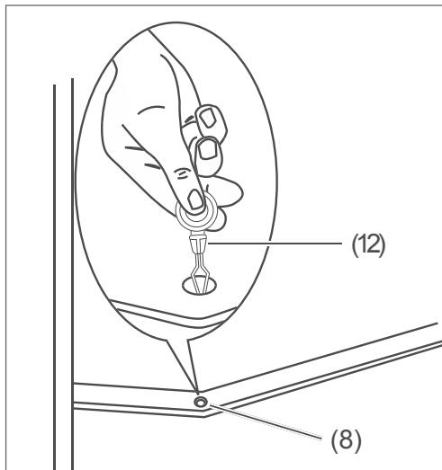
14. The defrost water drain (8) can be found on the rear wall of the refrigerator compartment above the vegetable drawer. Clean it regularly with the cleaning tool (12).
