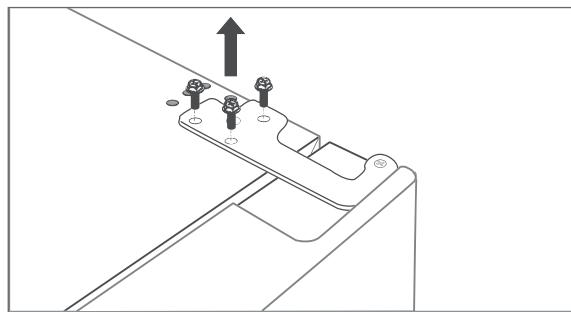
3. Unscrew the 3 screws on the upper hinge and remove the hinge.
