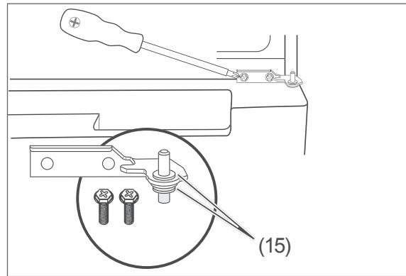
6. Unscrew the middle hinge and remove it. Pay attention to the plastic discs (15). They must later be repositioned correctly in the same place.
