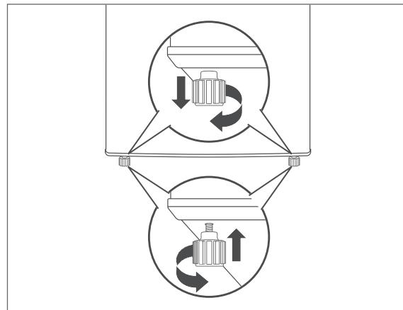
2. Level out any unevenness on the ground using both of the front screw feet.
