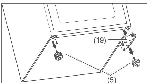
10. Tilt the unit slightly backwards against a wall so that the lower hinge (19) is accessible.
