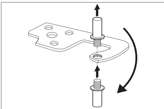
17. Use a pair of pliers to unscrew the hinge pin and screw it back in on the other side of the hinge plate.
