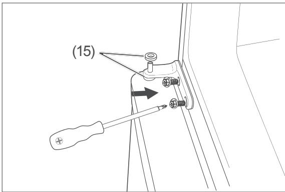
16. Reinsert the middle hinge into the new position. In the process, pay attention to the two plastic discs (15). Screw the hinge tight.
