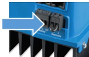
Remote connector with wire loop
