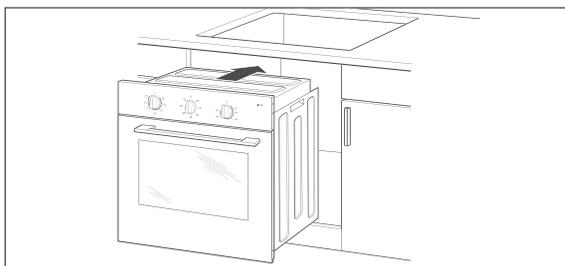
1. Push the oven into the recess until the front fascia is flush with the installation unit. The mains connection must not be kinked, pinched or otherwise damaged.
