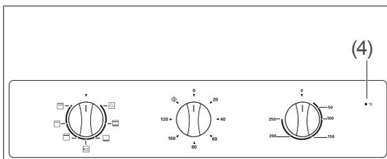
The red temperature indicator light (4) will light up as soon as you have selected a heating method and set the temperature and timer (2). It will light up while the oven is heating up and/
