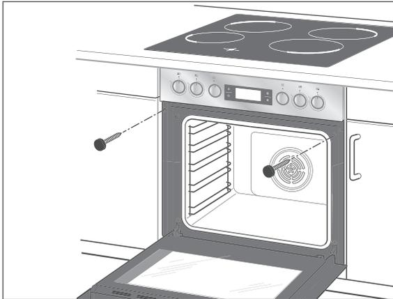
6. Screw the oven to the built-in cabinet with the two screws which have been supplied.
