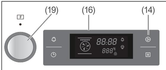
1. Selecting a function: Turn the dial (19) until the display (16) shows the corresponding symbol and its standard temperature.
