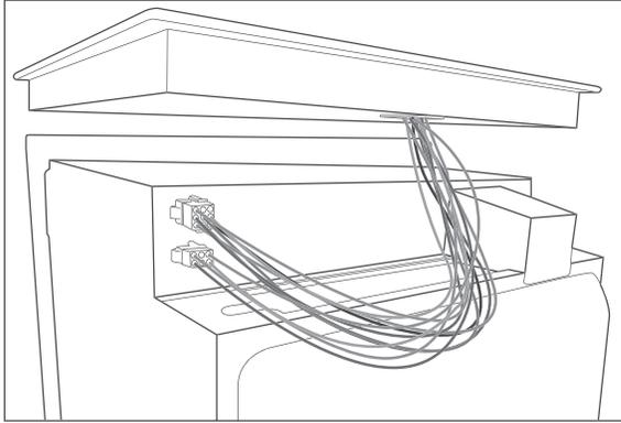
3. Insert the hob plugs into the sockets on the back of the oven. Do not use any force. The plugs are coded. Polarity reversal is therefore not possible.
