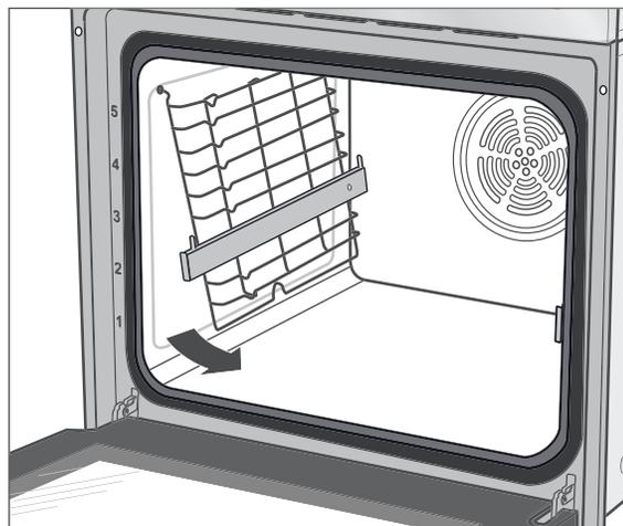
2. Pull the bottom of the oven rack guide approx. 45° away from the wall so that you can remove it.
