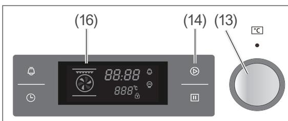
5. Adjusting the temperature: Turn the dial (13) until the display (16) shows the desired temperature.
