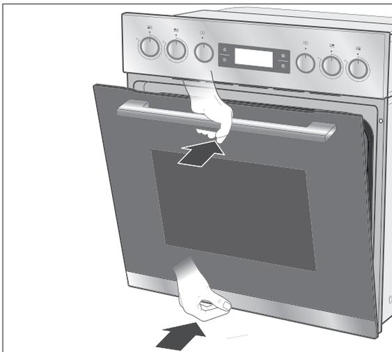
4. With both hands, lightly lift and guide the door forward out of its hinges.
