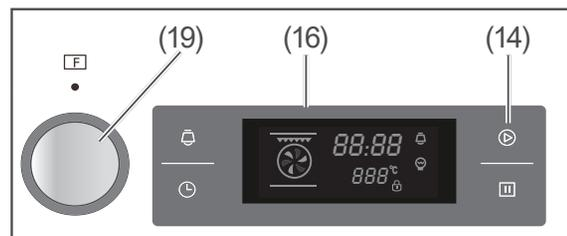
1. Selecting a function: Turn the dial (19) until the display (16) shows the
