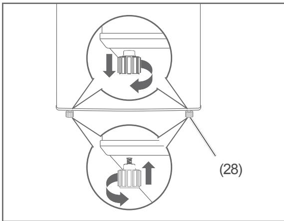
4. Level out any unevenness on the ground using the two front screw feet (28).
