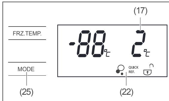
Select the setting (22) QUICKREF. "Quick refrigerating", for example when you would like a can you have put in the fridge to be cooled faster.
