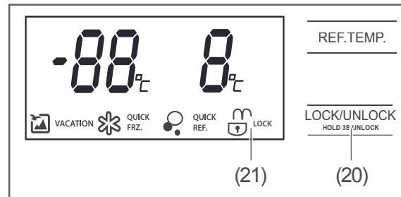
The fridge-freezer is protected against unintentional changes in settings. The symbol lights up on the display. If any button is pressed you will hear a beeping sound and the display (21) will flash. The control panel is locked.
