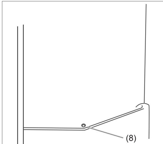
10. The defrost water drain (8) can be found on the rear wall of the refrigerator compartment above the vegetable drawer. If necessary, clean it e.g. with a toothpick.
