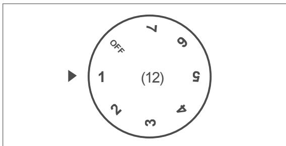
1. Set the temperature controller (12) to a setting of between "1" and "7".
