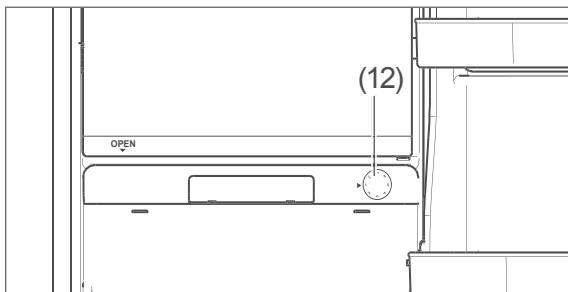
The temperature controller (12) is also used to switch the appliance on and off. It is located on the right below the freezer compartment and can be freely adjusted.
