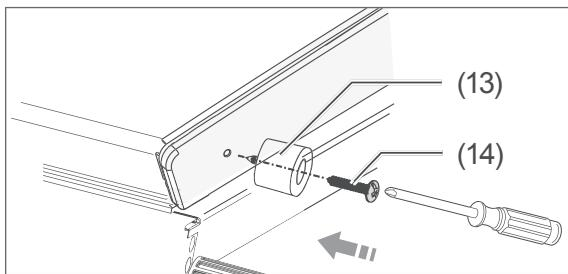
5. Screw the enclosed support leg (13) to the bottom edge of the appliance door using the enclosed screw (14).
