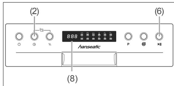
The wash cycle normally starts as soon as you press the ‘Start/Pause’ button (6). If you want the cycle to begin later, you can specify this. The start time can be delayed between 1 and 24 hours.
