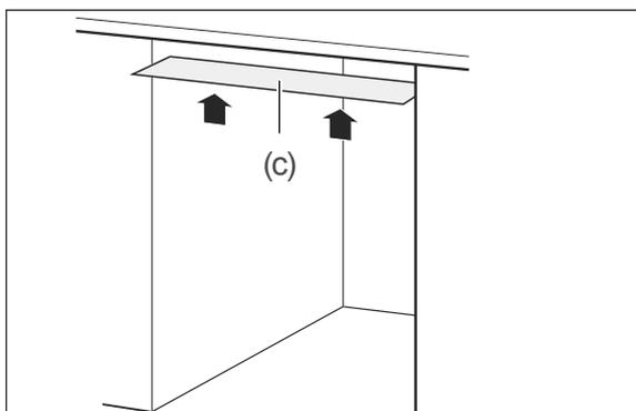
3. Affix the condensation protection film supplied (c) to the underside of the worktop. In this way, you will avoid damage to the work surface as a result of hot steam which may be emitted from the dishwasher if the dishwasher door is left open.
