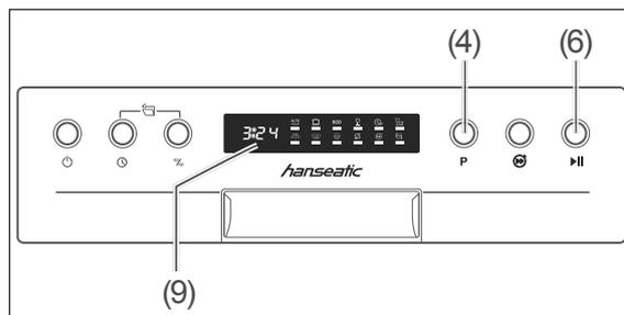
1. Press the button ▶II (6) in order to interrupt the dishwashing programme. The remaining duration display (9) will remain permanently illuminated.
