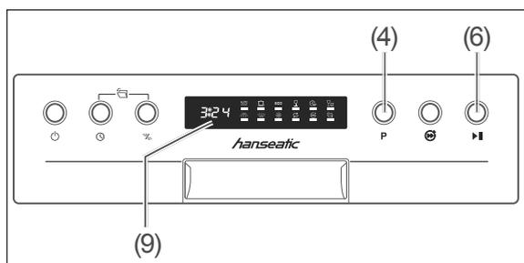
You can interrupt an active dishwashing programme at any point and start a new one. However, do not forget to add extra dishwasher detergent if the programme has already been running for a longer period and the cover of the dishwasher detergent compartment is already open.
