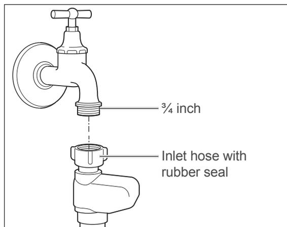
For water supply, you need a water tap with a  $\frac{3}{4}$  inch screw connector.
