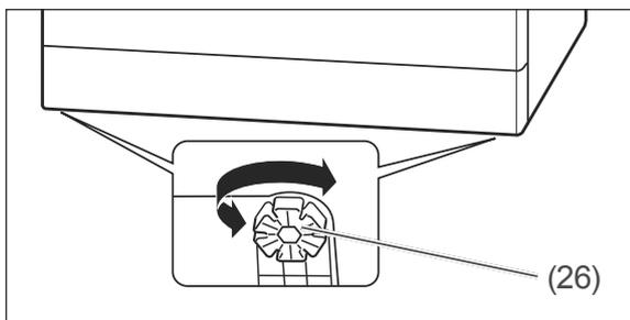
5. In order to equalise unevenness in the floor and set up the dishwasher on a level horizontal base, you can screw the four appliance feet (26) in or out. There are slots in the appliance feet around the circumference. Insert a screwdriver and turn the appliance foot. Use a spirit level to set up the dishwasher.
