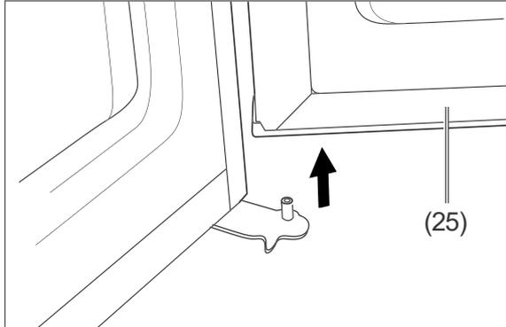
9. Open the freezer door (25), remove it and place it to one side.
