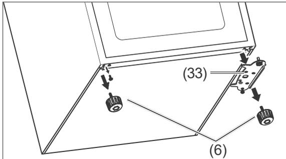
10. Tilt the unit slightly backwards against a wall so that the lower hinge (33) is accessible.
