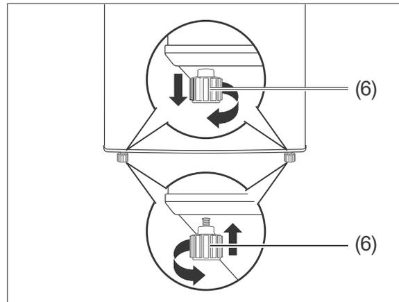
2. Level out any unevenness on the ground using both of the front screw feet (6).
