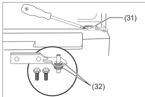
8. Unscrew the middle hinge (31) and remove it. Pay attention to the plastic discs (32). These must later be repositioned correctly in the same place.
