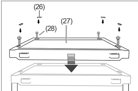
6. Screw the appliance cover (27) in place using the screws (28), and replace the protective covers (26).
