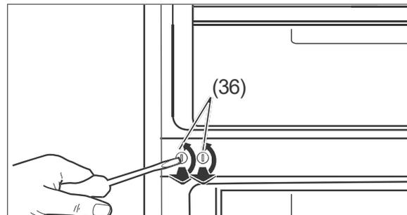
4. Using a flat-tip screwdriver, turn the two dummy plugs (36) until the slits are in a vertical position, at which point they can be removed.
