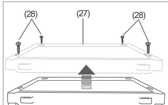
4. Using a Phillips screwdriver, loosen the retaining screws (28) before removing the appliance cover (27).
