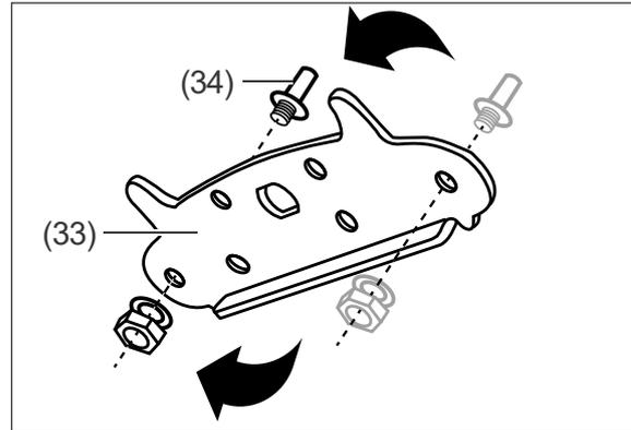
1. Reposition the hinge pin (34) belonging to the hinge (33) as displayed above.
