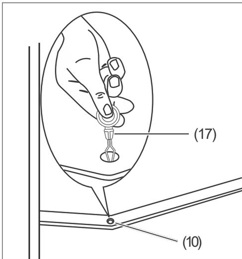
14. The defrost water drain (10) can be found on the rear wall of the refrigerator compartment above the vegetable drawer. Clean it regularly with the cleaning tool (17).
