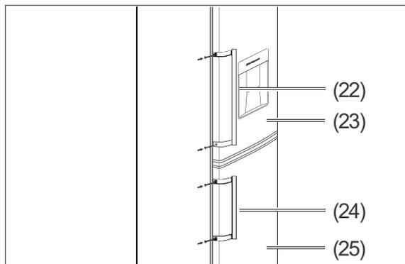
2. Affix the larger handle (21) to the fridge door (22) using the screws (23), and attach the smaller handle (24) to the freezer door (25).
