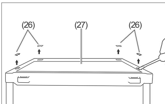
3. Using a flat-tip screwdriver, lift out the protective covers (26) found on the appliance cover.
