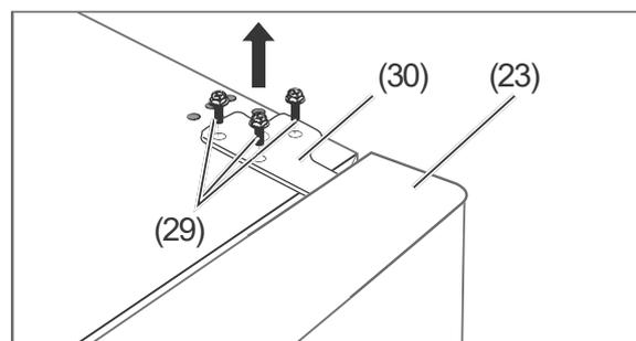
5. Unscrew the 3 screws (29) located on the upper hinge (30).
