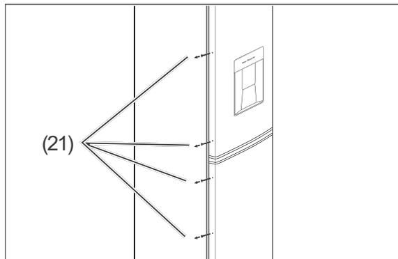
1. Loosen the screws (21) situated on the sides of the doors using a Phillips screw-driver.
