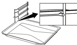
**Proper placement of the wire grill and tray on the telescopic rails-On models with wire shelves and telescopic models**
