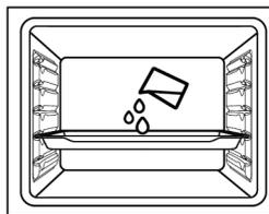
3. Set the oven to the easy steam cleaning operating mode and operate it at 100°C for 15 minutes.
