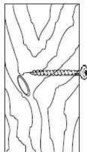
**Wood** If fixing to wood make sure that it isn't chipboard as screws can easily pull away from the core structure
