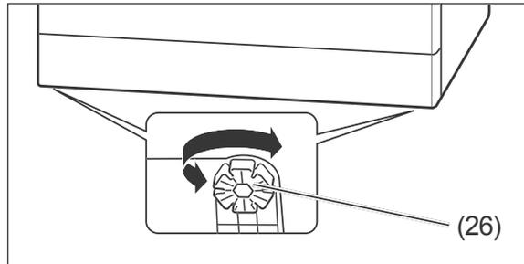
3. In order to equalise unevenness in the floor and set up the dishwasher on a level horizontal base, you can screw the four appliance feet (26) in or out. There are slots in the appliance feet around the circumference. Insert a screwdriver and turn the appliance foot. Use a spirit level to set up the dishwasher.
