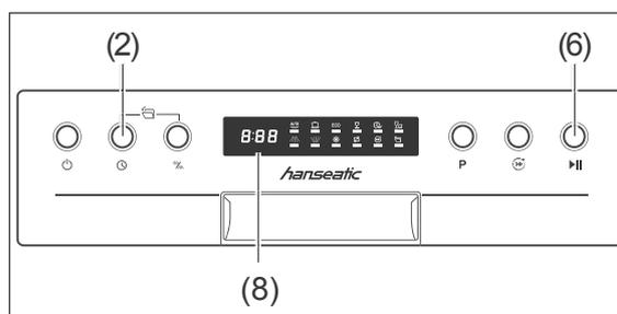
The wash cycle normally starts as soon as you press the ‘Start/Pause’ button (6). If you want the cycle to begin later, you can specify this. The start time can be delayed between 1 and 24 hours.
