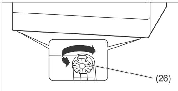
5. In order to equalise unevenness in the floor and set up the dishwasher on a level horizontal base, you can screw the four appliance feet (26) in or out. There are slots in the appliance feet around the circumference. Insert a screwdriver and turn the appliance foot. Use a spirit level to set up the dishwasher.
