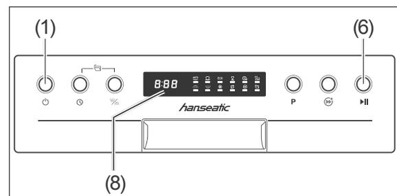
3. If the dishwasher is switched on, switch it off with the button  $\odot$  (1).
