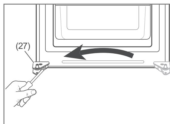
22. Screw the lower hinge (27) onto the opposite side.
