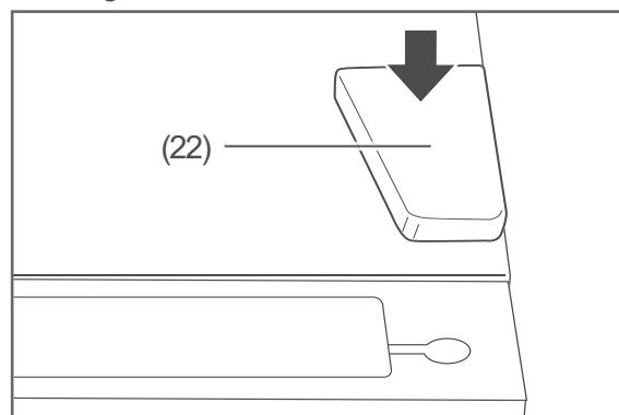
6. Reinsert the blanking plate (22) opposite the hinge side.
