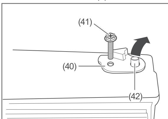
3. Loosen the screw (41) and remove the metal reinforcement (40) and the plastic sleeve (42).
