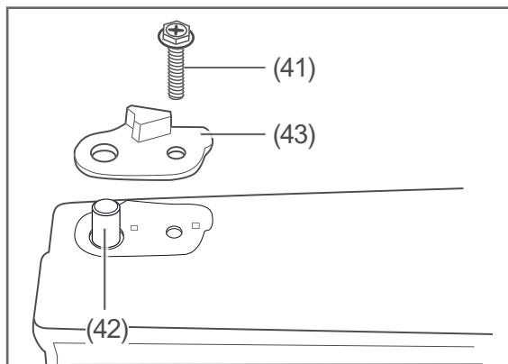
4. Insert the plastic sleeve (42) on the opposite side and use the screw (41) to screw the supplied metal reinforcement (43) on the opposite side.
