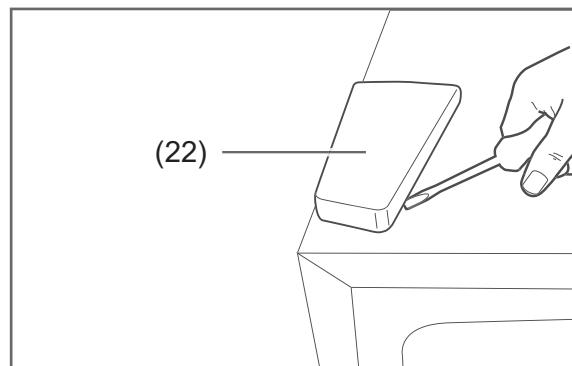
4. Lever the opposite blanking plate (22) upwards also and lift it off.
