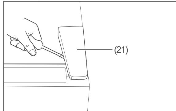
3. Gently lever the blanking plate (21) on the upper door upwards with a flat-headed screwdriver and lift it off. Store the blanking plate in a safe place.
