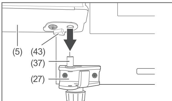
1. Reattach the freezer door (5) so that the pin screw (37) on the lower hinge (27) slides into the hole (43) in the metal reinforcement.
