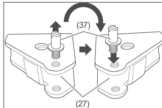
21. Unscrew the pin screw (37), turn the lower hinge over (27) and tighten the pin screw on the other side.
