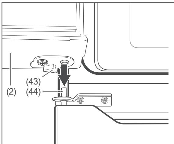
Reattach the fridge door (2) so that the top of the pin (44) slides into the hole in the metal reinforcement (43).
