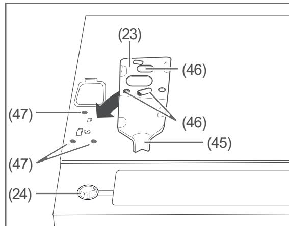
4. Insert the upper hinge (23) so that the hinge pin (45) slides into the plastic insert (24) and the screw holes (46) lay over the holes (47) in the appliance casing.
