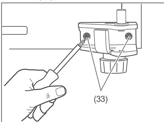
18. Unscrew both screws (33), and remove the lower hinge (27).
