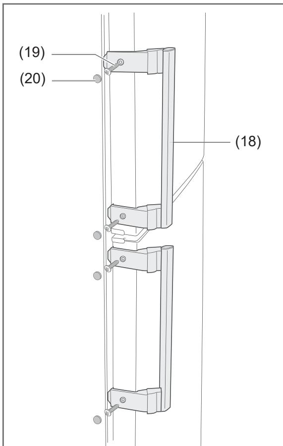
2. Attach the door handles (18) to both doors using the enclosed screws (19).
