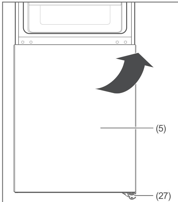
11. Lift the freezer door (5) out of the lower hinge (27), and remove it.
