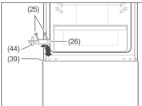
2. Reinsert the middle hinge (26) so that the lower part of the pin (44) slides into the insert (39).
