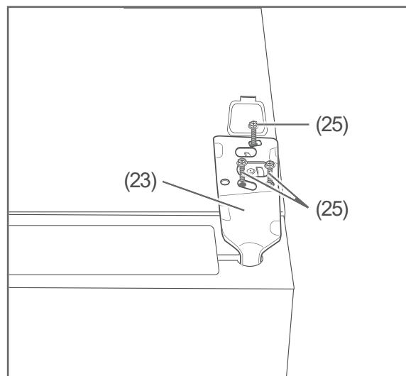
5. Loosen the three screws (25) of the top hinge (23), remove them and keep them in a safe place.
