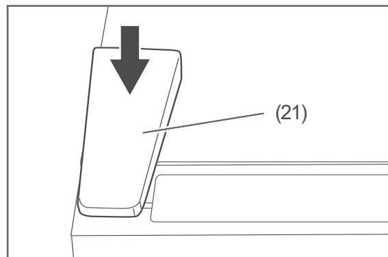
5. Reinsert the blanking plate (21) on the hinge side.
