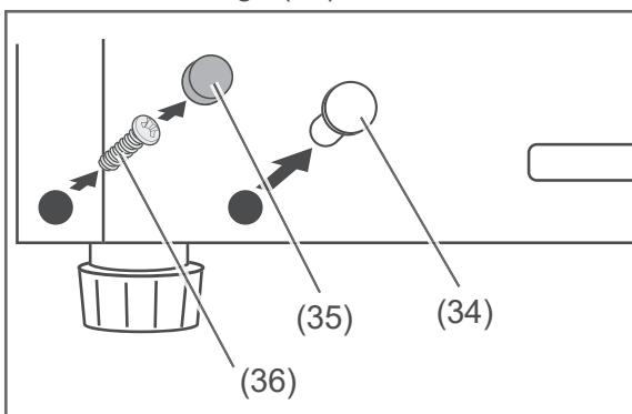
19. Lever out the blind plugs (34) and the cover cap (35) and loosen the screw (36).
