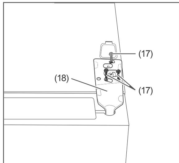
5. Loosen the three screws (17) of the top hinge (18), remove them and keep them in a safe place.
