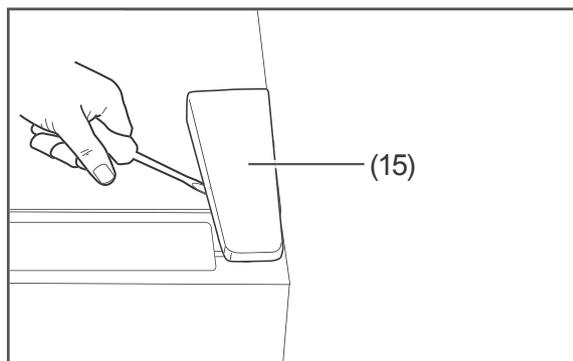
3. Gently lever the blanking plate (15) on the upper door upwards with a flat-headed screwdriver and lift it off. Store the blanking plate in a safe place.
