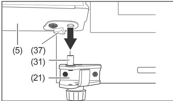
1. Reattach the freezer door (5) so that the pin screw (31) on the lower hinge (21) slides into the hole (37) in the metal reinforcement.
