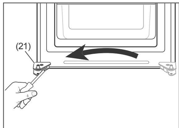
22. Screw the lower hinge (21) onto the opposite side.
