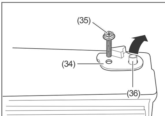
3. Loosen the screw (35) and remove the metal reinforcement (34) and the plastic sleeve (36).
