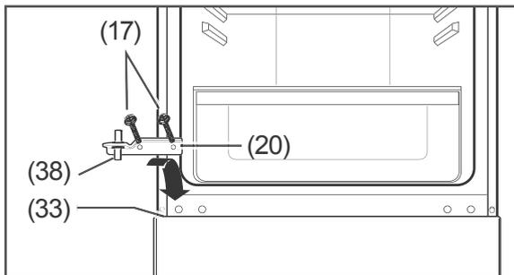
2. Reinsert the middle hinge (20) so that the lower part of the pin (38) slides into the insert (33).
