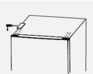
20. Loosen the pin of the upper hinge and turn the hinge 180°.
