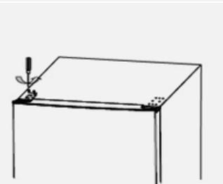
24. If necessary, readjust the hinges and fit the cover cap at the top right.
