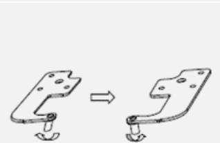
22. Fasten the hinge to the upper left side of the appliance with the two screws.
