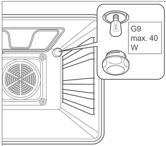
3. Unscrew the glass cover anticlockwise and remove it.
