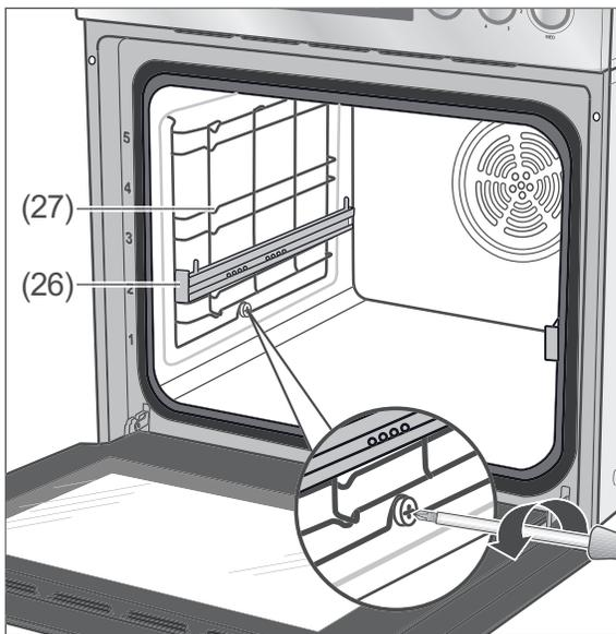
1. Loosen the screws of the oven rack guides and remove them.
