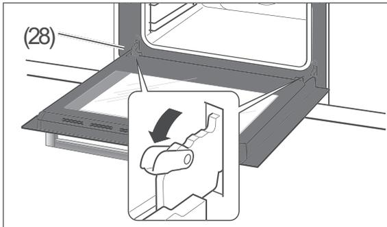
2. Fold the clips (28) on both sides all the way forward. Use a screwdriver if necessary.
