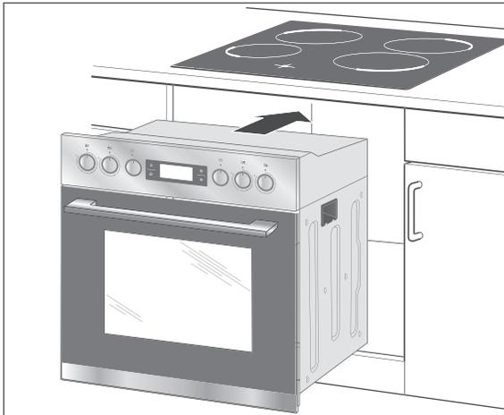
2. Use the carrying handles on the side of the oven to lift it and then push it as far back into the built-in cabinet so that the connections and earthing screw for the hob can still be easily reached.
