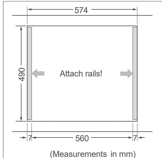
3. Attach adjustment strips to the left and to the right of the worktop in order to achieve the width of 560 mm.
