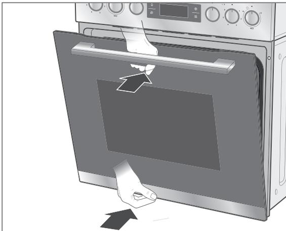
4. With both hands, lightly lift and guide the door forward out of its hinges.
