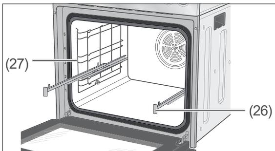
The side walls of the cooking compartment are equipped with oven rack guides (27) with telescopic oven rails (26). These make it eas-
