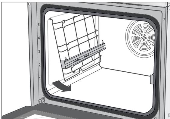
2. Pull the bottom of the oven rack guide approx. 45° away from the wall so that you can remove it.
