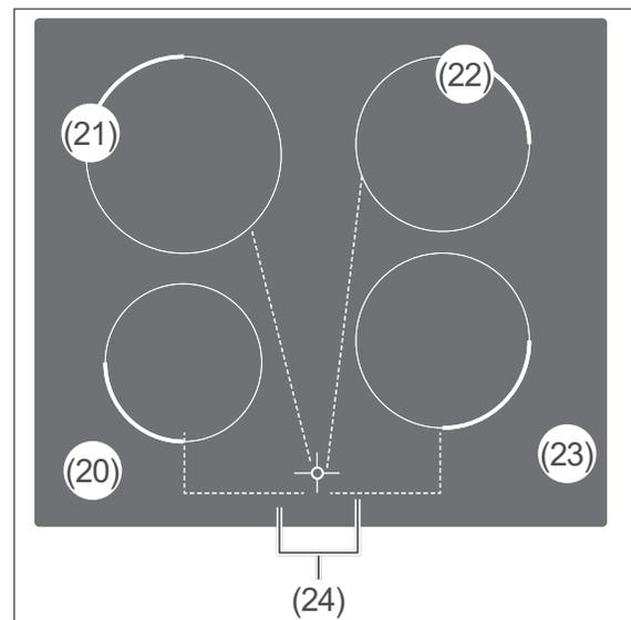
The residual heat indicators (24) indicate that surfaces are hot to prevent you from burning yourself. The H symbol indicates which of the cooking zones are hot.
