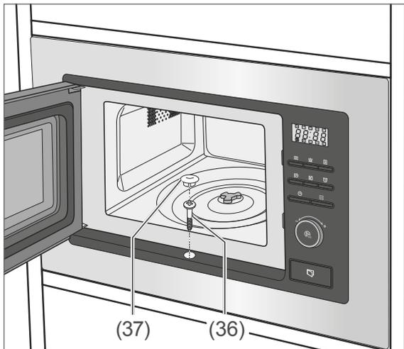
6. Secure the appliance in the hole with the supplied screw (36) and cover the screw with the cover (37).
