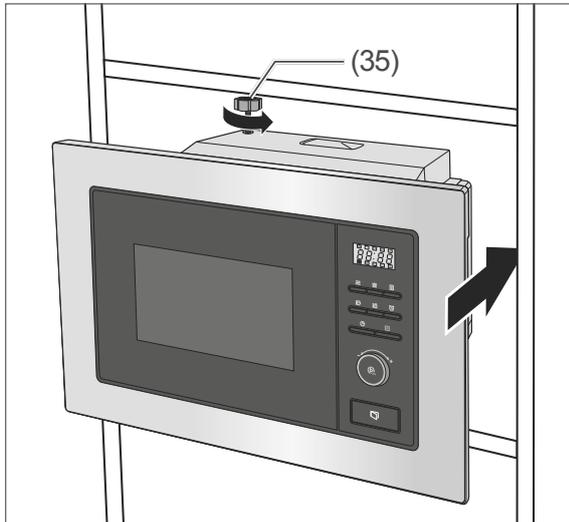
4. Adjust the fixing screw to leave a distance of approx. 1 mm between the installation compartment and the fixing screw.
