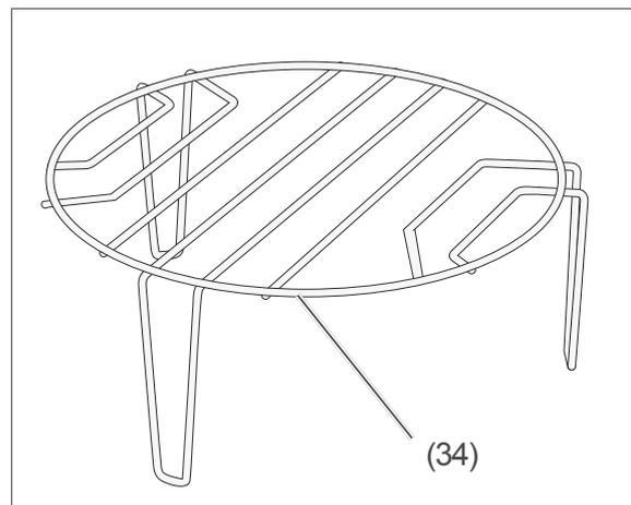
The grill rack (34) is not suitable for microwave mode. This can cause sparks. Use the grill rack exclusively in purely grill mode or in microwave-combi mode [ - 1 and [ - 2.
