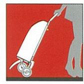
Try to keep the trolley as upright as possible. The ease of movement is reduced or increased according to the angle of inclination.
