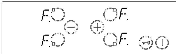
If residual heat is present, 'H' will be displayed in the appropriate heater displays.
