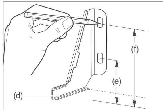
4. Position the tilt protection (d) on the line on the wall such that the side with the holes lies flat against the wall and the protruding limb fits into the slot on the cooker.
