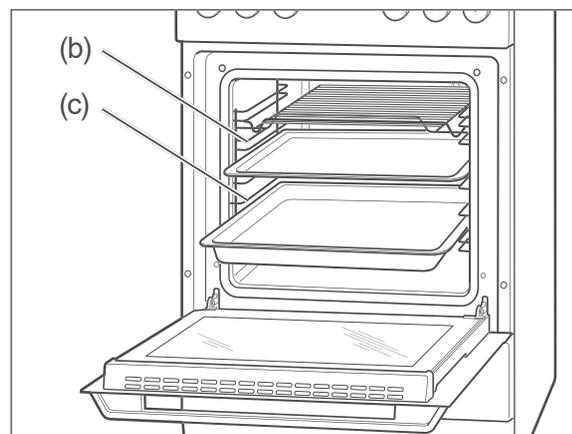
The supplied baking tray (b) and the dripping pan (c) both have an angled edge. Please ensure that this edge is facing forward on being placed in the oven.
