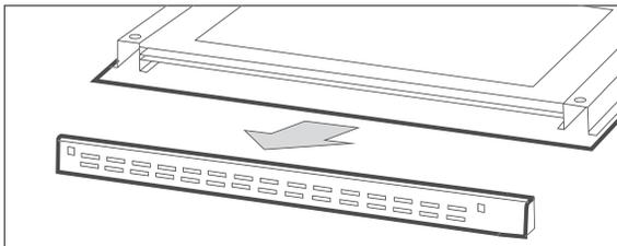
3. Carefully removed the metal grid.
