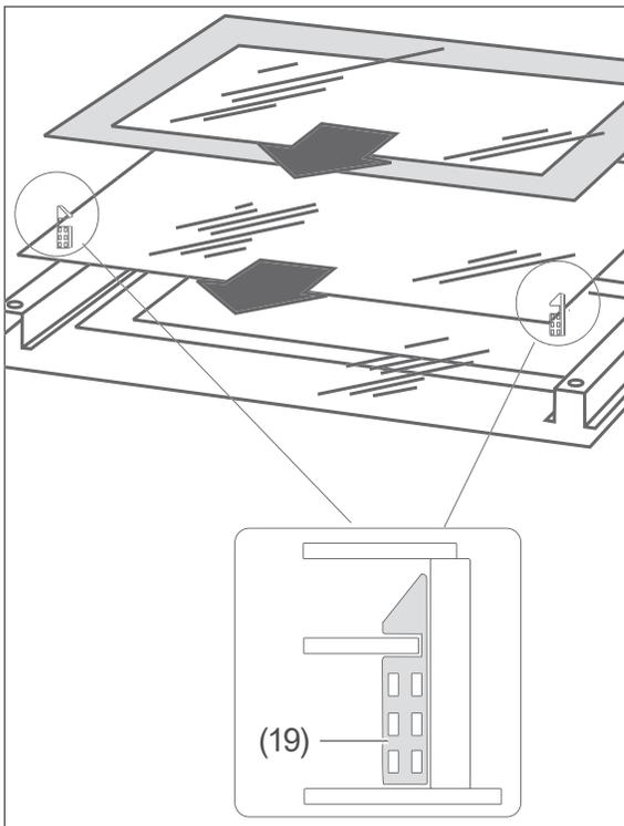
4. Remove the upper pane from the mounts below the hinges and carefully set it down.
