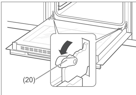
2. Fold the clips (20) on both sides all the way forward. Use a screwdriver if necessary.
