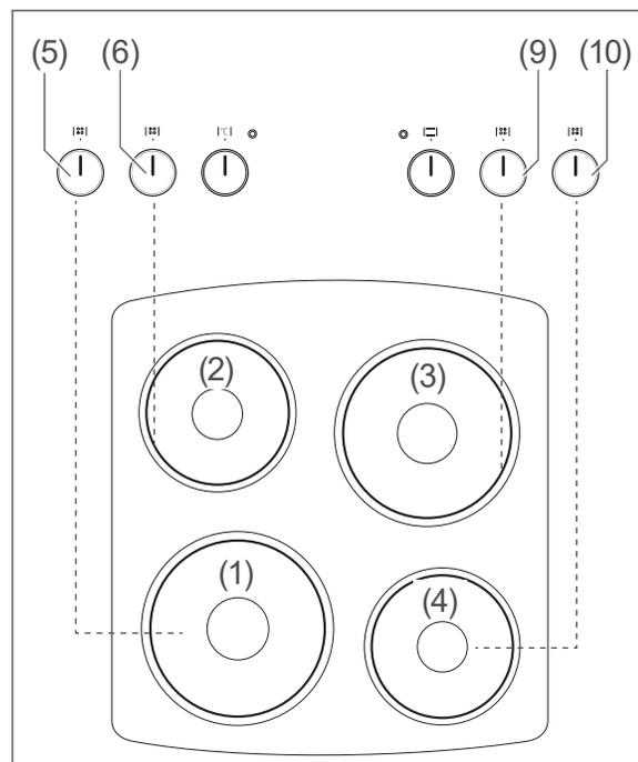
The cast-iron hob has two turbo and two ‘normal’ solid plates. The turbo solid plate has a red cross in the middle; this disappears with increased use. The turbo solid plate operates like normal solid plates, but they are more powerful and heat up quicker.
