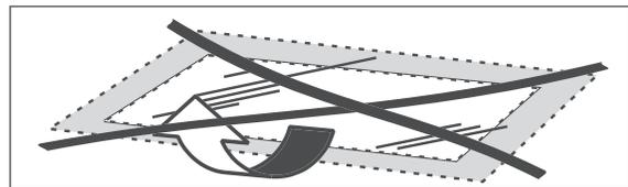
11. Reposition the upper pane in the mounts at the hinges. Make sure that the smooth side is facing outwards.
