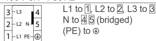
L1 – L3: Phase(s), N: Neutral conductor, PE: Protective conductor (earth wire)
