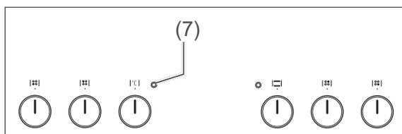
The red oven light (7) will illuminate as soon as you have selected a heating method and set the temperature. It will light up while the oven is heating up and/or re-heating. Once it goes out, the set oven temperature has been reached.
