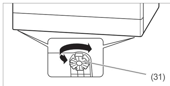
3. In order to compensate for uneven floor surfaces and set up the appliance horizontally, you can screw the four adjustable feet (31) in or out. The adjustable feet have slots around their circumference. Insert a screwdriver and turn the adjustable foot. Use a spirit level to set up the appliance.
