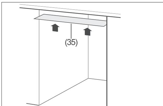
3. Affix the condensation protection film supplied (35) to the underside of the worktop. In this way, you will avoid damage to the worktop as a result of hot steam which may be emitted from the dishwasher if the dishwasher door is left open.
