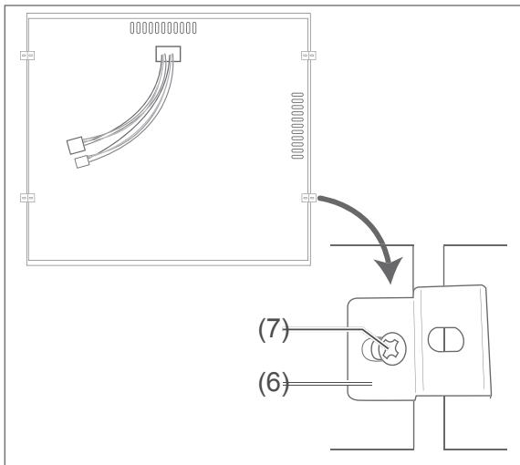
4. Use the supplied retaining clamps (6) and screws (7) to fix the hob in place to the worktop and to prevent it from slipping.
