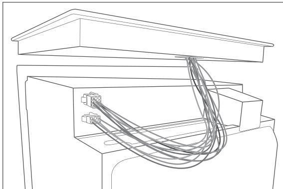
3. Insert the plugs of the hob into the sockets on the back of the cooker. Do not try to insert the plugs into the sockets with force. The plugs are coded. Polarity reversal is therefore not possible.
