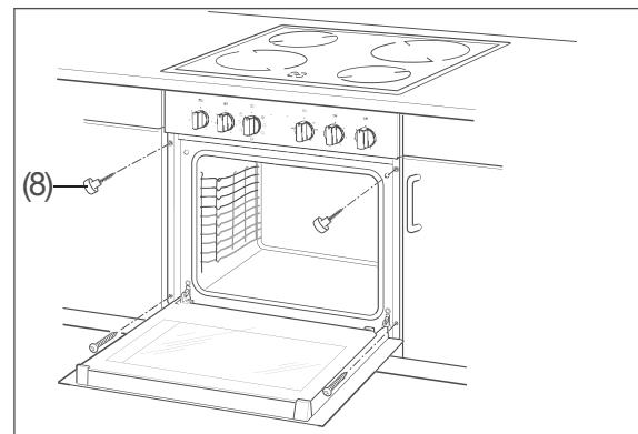
5. Screw the enclosed screws (8) through the holes on the sides of the oven into the sides of the built-in cabinet.
