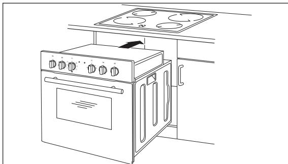
2. Position the oven in front of the built-in cabinet in such a way that the connection sockets for the hob remain accessible.
