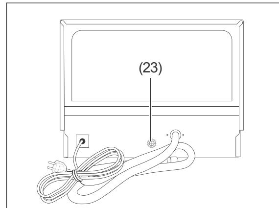
1. Screw the union nut of the inlet hose of the connection for the appliance (23) tight.
