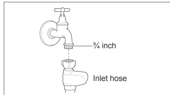
2. Screw the inlet hose's union nut with aqua stop to the tap hand-tight.
