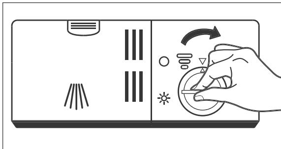
4. Insert the rinse aid dispenser catch (22) and give it a quarter turn clockwise. The markings on the lid and the rinse aid dispenser (22) must be aligned upon insertion.
