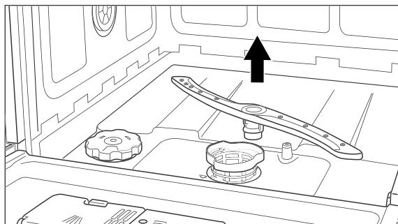
2. Pull the spraying arm (18) up and off.
