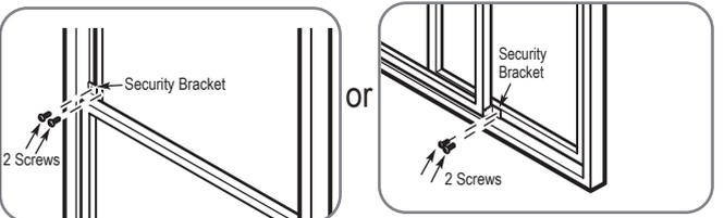
4. If desired, install the security bracket with 2 screws as shown.
