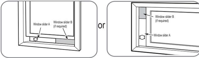
2. Insert the window slider assembly into the window opening.
