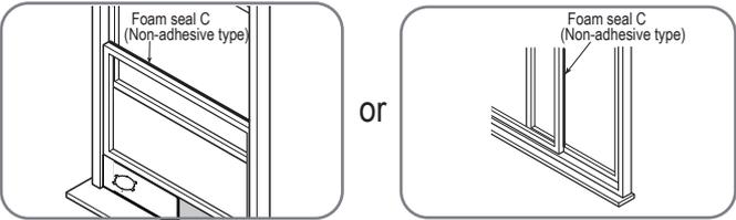
3. Cut the non-adhesive foam seal C strip to match the width of the window. Insert the seal between the glass and the window frame to prevent air and insects from getting into the room.
