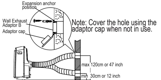
Note: To ensure proper function, DO NOT overextend or bend the hose. Make sure that there is no obstacle around the air outlet of the exhaust hose (in the range of 500mm) in order to the exhaust system works properly. All the illustrations in this manual are for explanation purpose only. Your air conditioner may be slightly different. The actual shape shall prevail.
