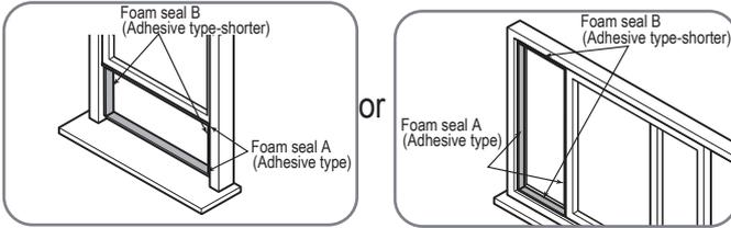
1. Cut the adhesive foam seal A and B strips to the proper lengths, and attach them to the window sash and frame as shown.
