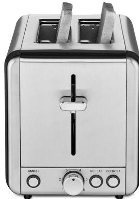
3. Select the desired degree of roasting with the roasting degree control (B). In position **1**, the roasting is lightest, in position **6**, it is darkest.
