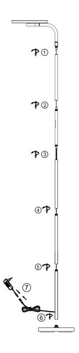
1. 2. 3. 4. 5. 6. Connect the pipes by rotating7. Plug it in to turn it on/ off.
