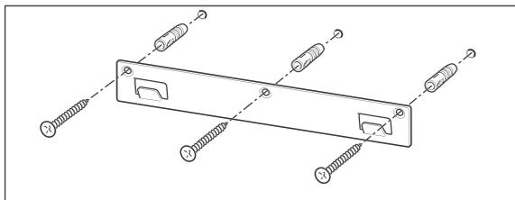
8. Insert the three dowels into the holes.
