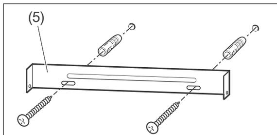
5. Screw the wall mount (5) to the wall with two screws.
