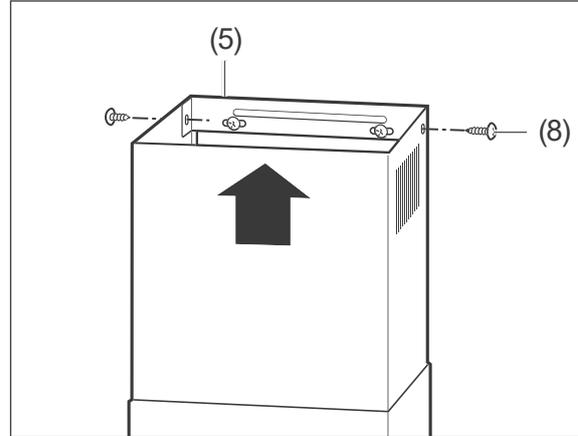
18. Pull up the upper part of the flue screen to the upper wall mount (5) and screw on the flue screen tightly with two screws (8).
