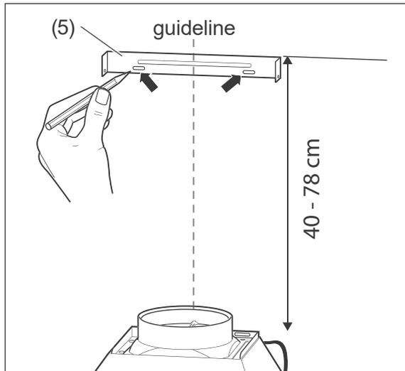
1. Hold the wall mount (5) horizontally against the wall at the desired flue height so that the centre of the wall mount aligns with the vertical guide line.
