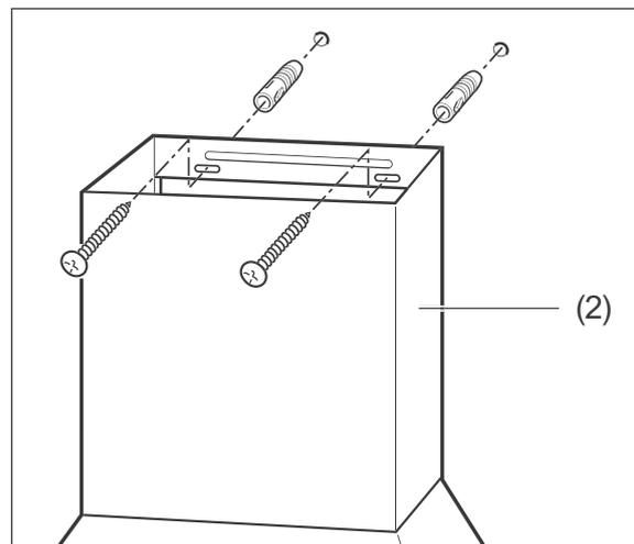
7. Place the flue screen (2) on the top of the exhaust hood.
