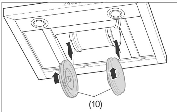
3. Only when replacing: Unscrew the old coal filter (10) from the motor and remove the activated charcoal filter.
