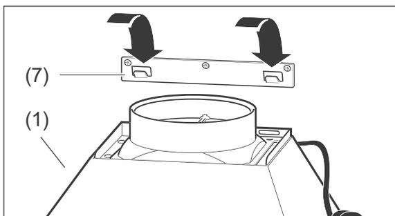
10. Hook the exhaust hood (1) carefully into the wall mount (7).
