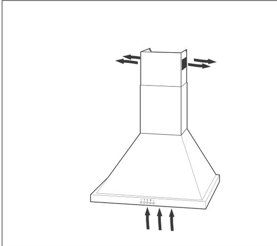
When air is circulated, the cooking fumes are sucked in and, following filtering, returned to the indoor air through the air outlets at the top of the appliance.
