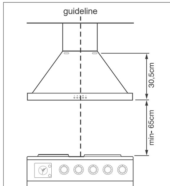
1. In order to place the appliance exactly over the centre of the stovetop, first use the pencil to draw a vertical guiding line on the wall. Ideally, use a level or a plumb bob from the ceiling of the room to the middle of the stovetop.
