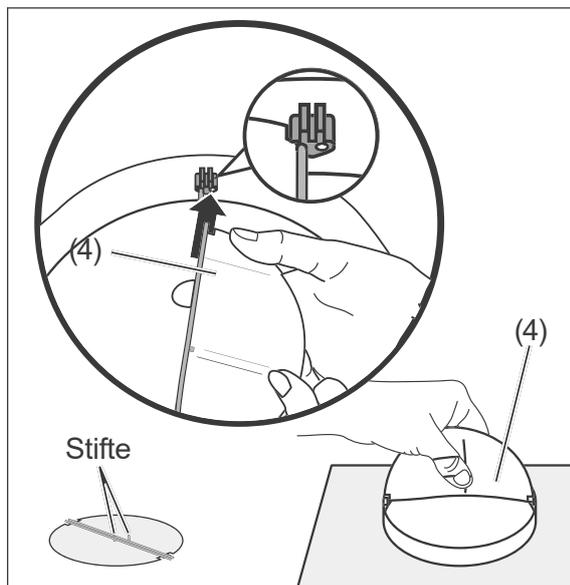
1. Place the two halves of the check valve (4) into the opening on the top of the Exhaust hood (1). Make sure that the pins on the valve are facing outwards.
