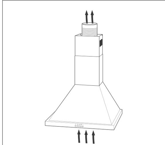
When air is extracted, the cooking fumes are sucked in, filtered through the grease filter, and released to the outdoors through the exhaust air hose.
