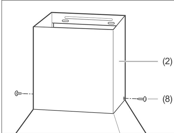
14. Screw the bottom of the flue screen (2) to the exhaust hood with two screws (8).
