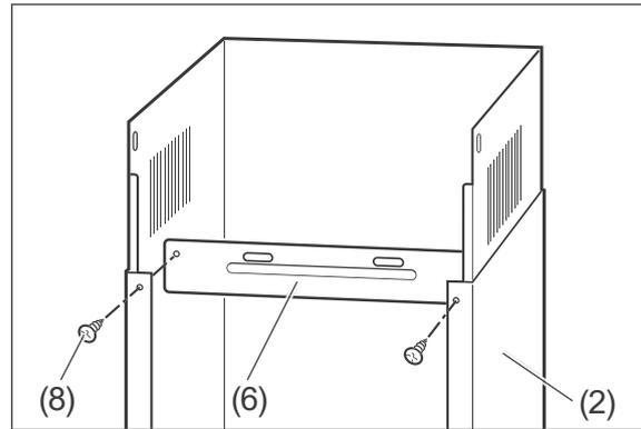
6. Screw the retaining plate (6) onto the lower half of the flue screen (2) with two screws (8).
