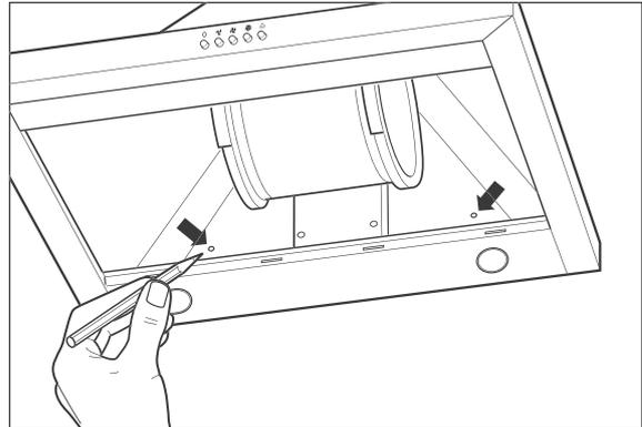
12. Draw the drill holes onto the wall through the openings inside the appliance.
