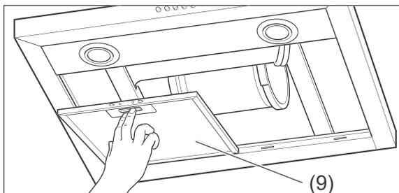
2. Push back the lock on the grease filters (9) and carefully remove the grease filters.
