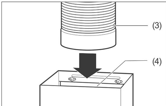
15. Only for exhaust air operation: Insert the end of the exhaust hose (3) with the larger diameter (153 mm) into the connection with the check valve (4).
