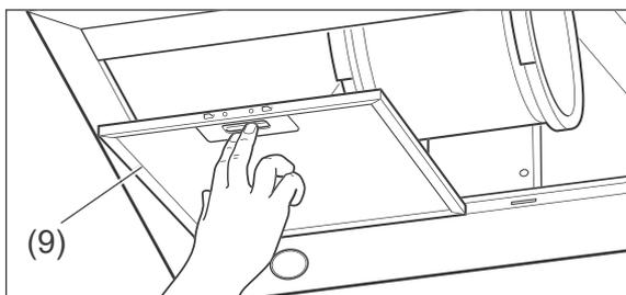
11. Push back the lock on the grease filters (9) and carefully remove the grease filters.
