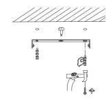
5. Put the washers and screws and tighten the screws.
