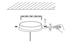
7. Screw the side screws into the metal base.
