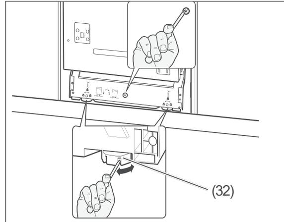
1. Insert a screwdriver into one of the slots and turn the adjustable feet to the height required.
