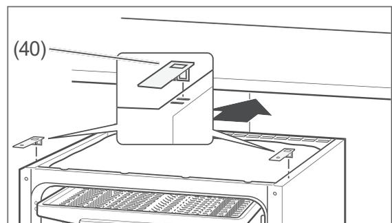
4. Insert the two mounting brackets (40) into the front slots on the top of the appliance so that you can screw the appliance to the worktop later on.
