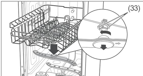
3. The upper spraying arm is affixed using a bayonet closure. To remove the spraying arm, hold the two serrated bayonet grips (33) still and turn the spraying arm clockwise.
