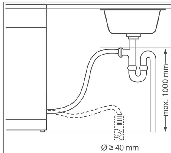
You can connect the end of the outlet hose in two different ways:
