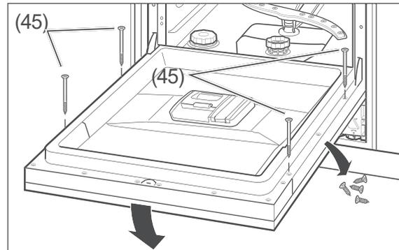
18. Remove the 4 screws from the inside of the door. Screw the front panel in place at these positions using the 4 enclosed screws (45).
