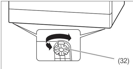
5. In order to compensate for uneven floor surfaces and set up the dishwasher horizontally, you can screw the four adjustable feet (32) in or out. The adjustable feet have slots around their circumference. Insert a screwdriver and turn the adjustable foot.
