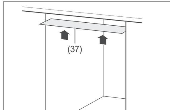
3. Affix the enclosed protective film (37) for condensation to the bottom of the worktop surface. In this way, you will avoid damage to the worktop as a result of hot steam which may be emitted from the dishwasher if the dishwasher door is left open.
