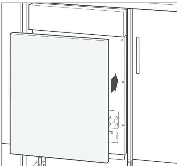
17. Attach the front panel to the appliance door of the dishwasher using the Velcro
