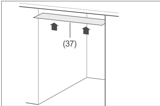
3. Affix the enclosed protective film (37) for condensation to the bottom of the worktop surface. In this way, you will avoid damage to the worktop caused by hot steam emitted from the dishwasher when the appliance door is left open.
