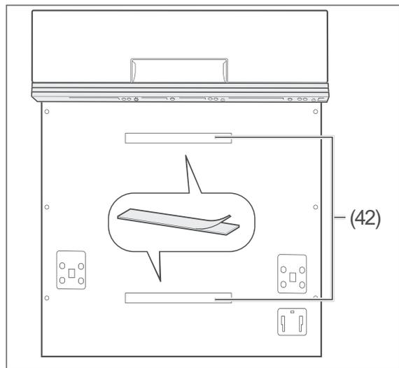
10. With the protective film removed, stick the Velcro strips onto the middle of the recessed areas on the appliance door.
