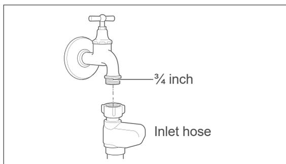
You will require a valve with a  $\frac{3}{4}$ -inch screw connector for the water supply.
