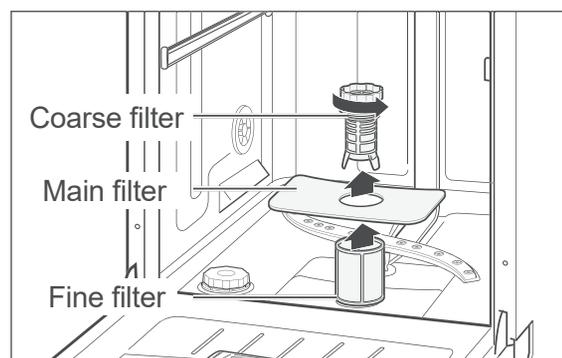
Check the coarse filter, the main filter and the fine filter after each rinse cycle and remove food residues and foreign bodies if necessary:
