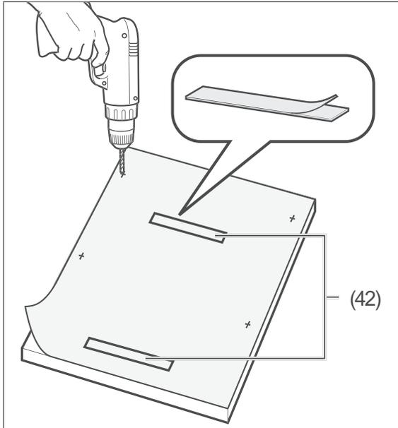
13. Lay the supplied drilling template on the reverse side of the front panel in such a way that the drilling template and the front panel are flush at the top.
