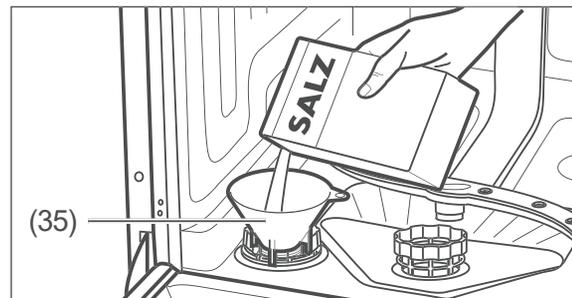
4. Place the supplied filling funnel (35) on the compartment opening.
