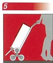
Try to keep the trolley as upright as possible. The ease of movement is reduced or increased according to the angle of inclination.
