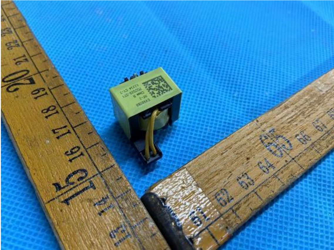
Picture 25. Top View of Transformer
