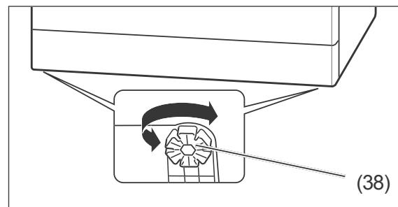
2. To equalise unevenness in the floor and set up the dishwasher on a level horizontal base, you can screw the two adjustable (38) feet in or out. The adjustable feet have slots around their circumference. Insert a screwdriver and turn the adjustable foot. Use a spirit level to set up the dishwasher.
