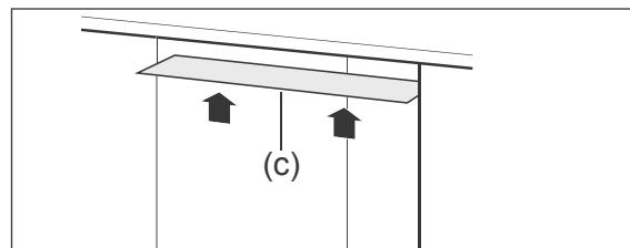
4. Affix the enclosed moisture barrier tape (c) to the underside of the worktop. In this way, you will avoid damage to the work surface as a result of hot steam which may be emitted from the dishwasher if the dishwasher door is left open.
