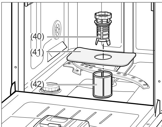
Check the coarse filter (40), the main filter (41) and the fine filter (42) after each rinse cycle and remove food residues and foreign bodies if necessary:
