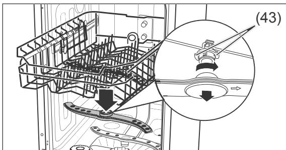
3. The upper spraying arm is affixed using a bayonet closure. To remove the spraying arm, hold the two serrated bayonet grips (43) still and turn the spraying arm clockwise.
