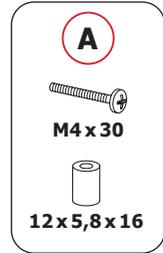
**Recessed surface installation: Put spacers between headplate and monitor. Install the upper two screws and don't screw them tight. Leave some space and hang the monitor on the head plate.**
