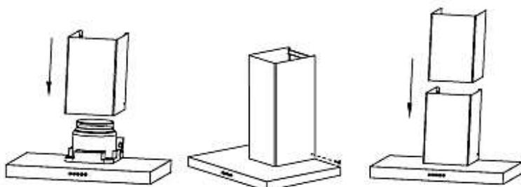
(9) Adjust the two chimneys relevant to the dimensions of the fixing bracket (s. fig. below).
