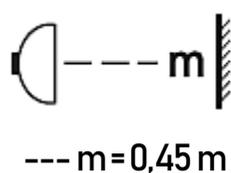
Required minimum distance to surfaces such as pot lids, oven cloths etc. to avoid any hot parts and risk of fire.
