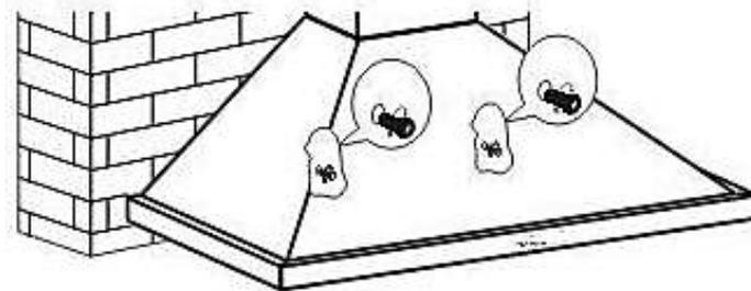
(3) Lift up the extractor hood and hang it on the wall bracket (s. fig. below). Fix the extractor hood by tightening the screws properly.
