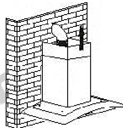
(7) Insert the inner chimney into the outer chimney (s. fig. below).
