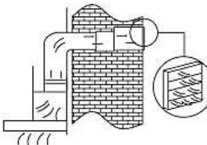
(8) Pull the inner chimney upwards and adjust it to the required height (s. fig. below).
