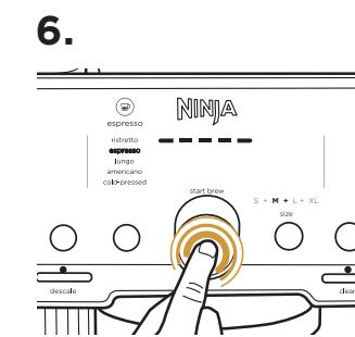
Press **START BREW**. The machine will beep to signal the brew has started. The progress bar will illuminate, indicating the status of the brew.
