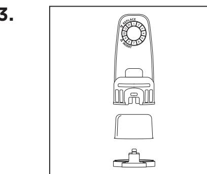
Remove end-cap from filter housing and insert filter. Clip end-cap back onto filter housing to secure filter in place.
