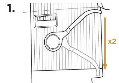
After grinding is complete, **push the integrated tamper lever down firmly until it stops**. You will feel some resistance as the puck compresses.
