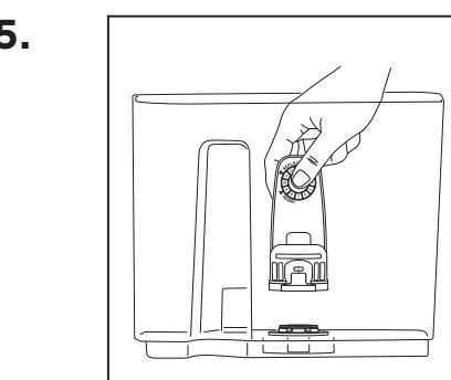
Install filter housing into reservoir.
