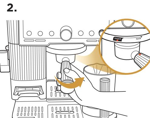
Fasten portafilter to align with lock arrow.
