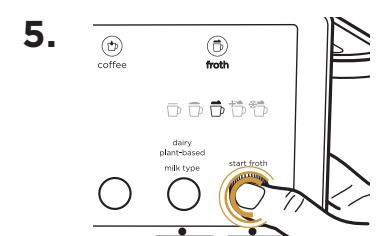
Press **START FROTH** to begin frothing. The machine will beep to signal the froth has started. The progress bar will illuminate, indicating the status of the froth.
