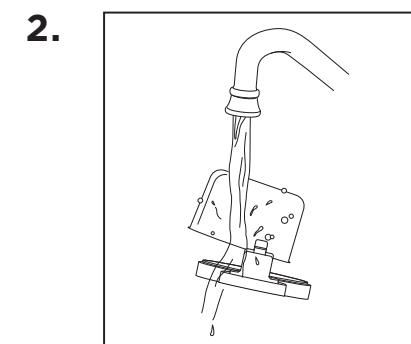
Rinse water filter and mesh for 60 seconds.
