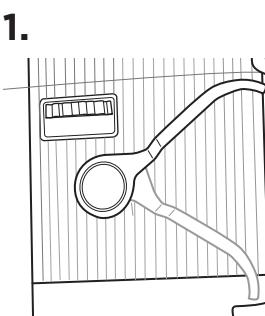
After grinding is complete, **push the integrated tamper lever down firmly until it stops**. You will feel some resistance as the puck compresses.
