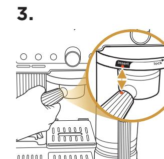
Place portafilter in group head (angled to the left) by aligning orange dot on portafilter with orange dot on group head.
