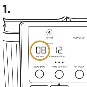
Check to see if the current grind setting matches the recommended setting.
