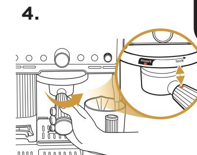
Fasten portafilter into group head until orange dot on portafilter aligns with lock arrow on group head.
