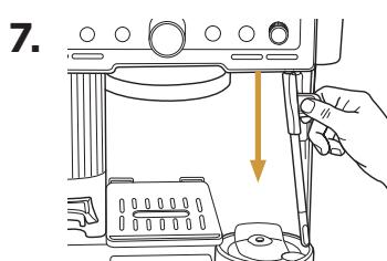
Push steam wand into its down position. The machine will automatically purge to clean inside of wand.
