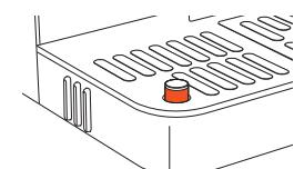
When the orange empty indicator rises enough to be visible, it's time to empty the main drip tray.
