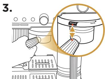
Place portafilter in group head (angled to the left) by aligning orange dot on portafilter with orange dot on group head.
