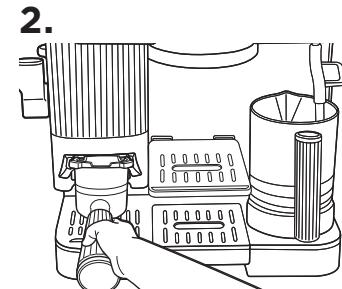
Insert the portafilter in the grinding cradle. Make sure it is level and fits securely. Once portafilter is installed in grinding cradle, it will be weighed. **To ensure accurate weight, let go of portafilter.**
