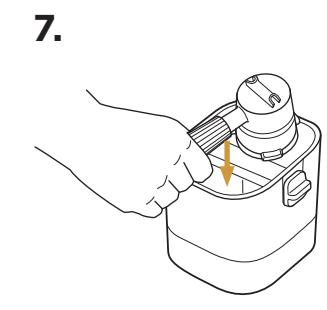
When finished, the machine will beep again to signify the brew is complete. Carefully remove portafilter from group head. Dispose of grounds by tapping the surface of the basket over a container or knock box.\*
