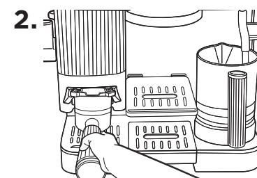
Insert the portafilter in the grinding cradle. Make sure it is level and fits securely. Once portafilter is installed in grinding cradle, it will be weighed. **To ensure accurate weight, let go of portafilter.**
