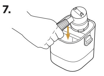
When finished, the machine will beep again to signify the brew is complete. Carefully remove portafilter from group head. Dispose of grounds by tapping the surface of the basket over a container or knock box.\*
