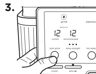
Press **START GRIND**. Do not touch portafilter until grinding is completed.
