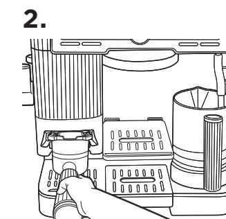
Release the tamper lever and remove the portafilter from the grinding cradle.
