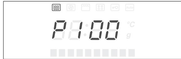
5. The indicator will illuminate on the display (2) and the power level indicator **P100** (=100 % microwave power) will be displayed.
