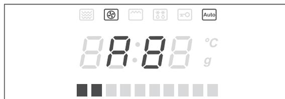
Pre-heating to 180 °C will start. The progress bar at the bottom of the display shows the heating progress.
