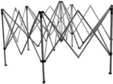
Pull out the support legs to the first stop. Release the ball stops by pressing on the ball and sliding the parts together or pulling them apart. The ball stops must click into place audibly.
