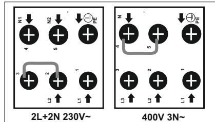
For the induction hob, the cable must be H05VV-F 5X2,5 mm<sup>2</sup> 60227 IEC 53
