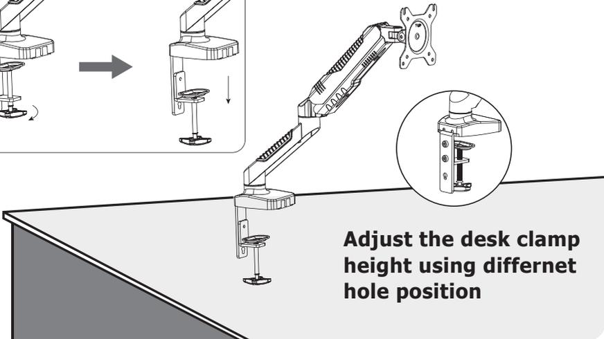
Tighten clamp using clamp screw until mount is securely fastened to desk.
