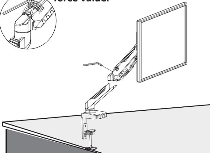
**Use a hex wrench to adjust the height tension of the gas spring arm, to keep different weight of monitors still at any position.**
