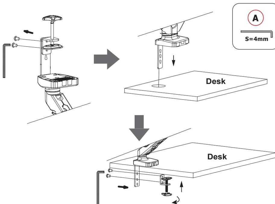
**Loosen the two screws on the base, pass it through the hole in the table, and screw in the two screws that have just loosened.**
