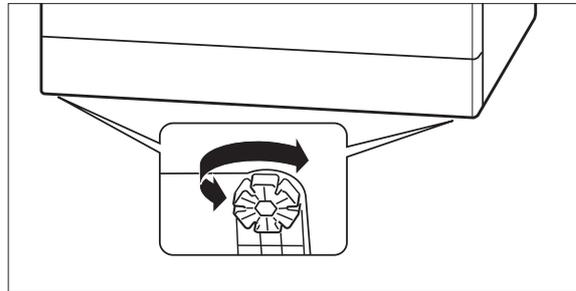
3. In order to equalise unevenness in the floor and set up the dishwasher on a level horizontal base, you can screw the four adjustable feet in or out. There are slots in the appliance feet around the circumference. Insert a screwdriver and turn the appliance foot.
