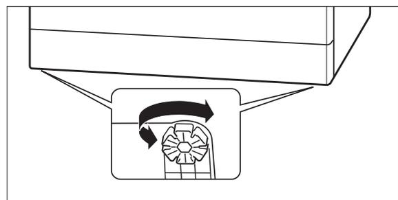
5. In order to equalise unevenness in the floor and set up the dishwasher on a level horizontal base, you can screw the four adjustable feet in or out. There are slots in the appliance feet around the circumference. Insert a screwdriver and turn the appliance foot.
