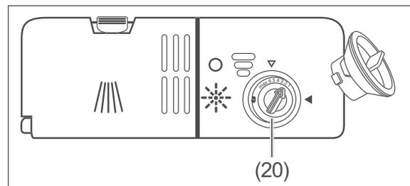
1. Turn the cover of the dishwasher salt compartment (20) a quarter turn in an anti-clockwise direction and remove it.
