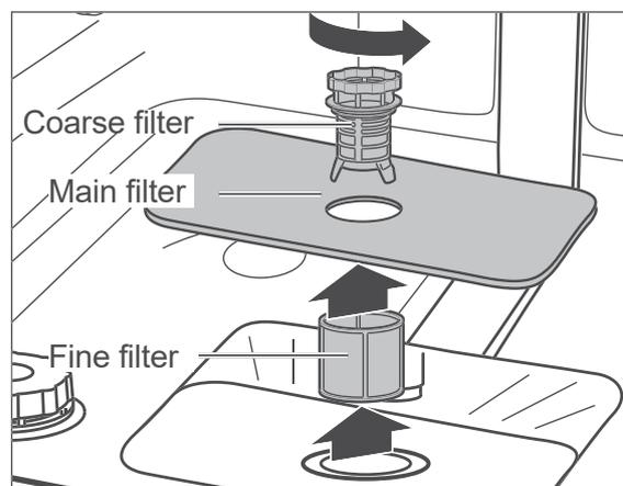
Remove any food scraps out of the coarse filter, the main filter and the fine filter.
