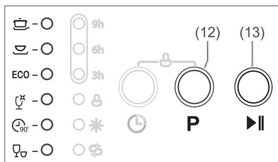
2. Press the **P** button (12) repeatedly until the LED to the right of the desired programme symbol lights up.
