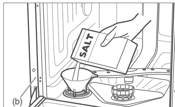
4. Place the supplied filling funnel (b) on the compartment opening.
