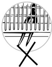
When loading the cutlery, ensure that it does not go through the bottom of the cutlery basket. Otherwise, the lower spraying arm will be blocked.
