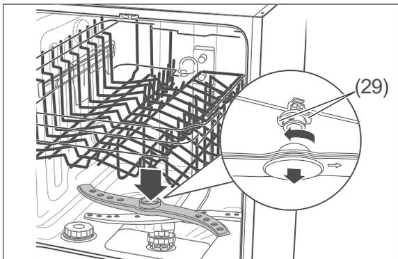
3. The upper spraying arm is affixed using a bayonet closure. To remove the spraying arm, hold the two serrated bayonet grips (29) still and turn the spraying arm clockwise.
