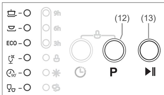
You can interrupt an active dishwasher programme at any point and start a new one. However, do not forget to add extra dishwasher detergent if the programme has already been running for a longer period and the cover of the dishwasher detergent compartment is already open.
