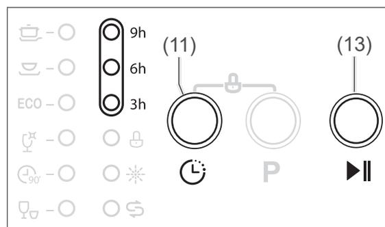
1. Press the “Delayed start” button (11) repeatedly until the LED to the left of the desired delay lights up.
