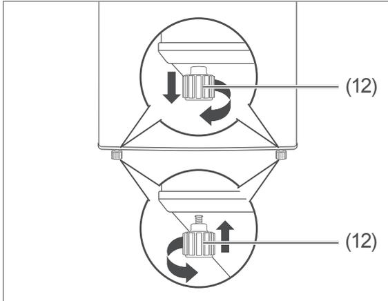
5. Level out any unevenness on the ground using both of the front screw feet (12).
